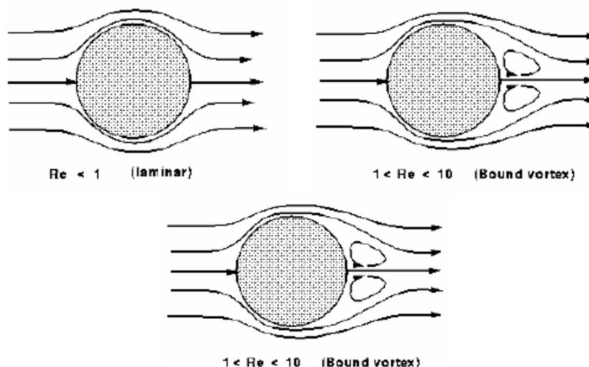
Fig. 1. Reynolds number on flow pass a cylinder [16]
