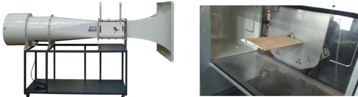
(a) AF100 Subsonic Wind Tunnel test setup
