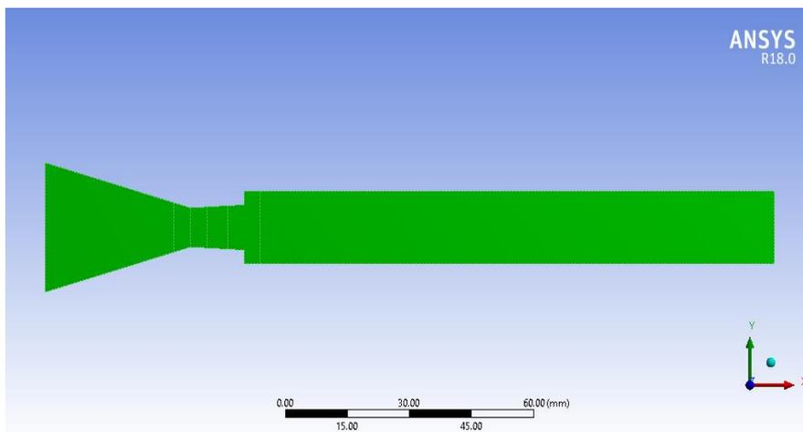
**Fig. 2.** Finite Element Model 2D planar CD nozzle for Area Ratio 2.56
