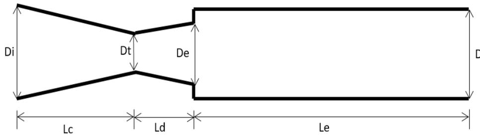
**Fig. 1.** FE Design of CD Nozzle with Suddenly Expanded Duct
