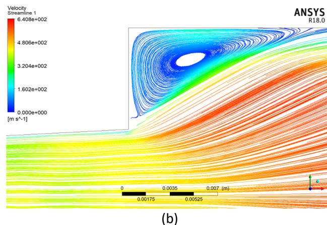
**Fig. 10.** Velocity Streamline for Area Ratio 6.25 (a) With Control (b) Without Control
