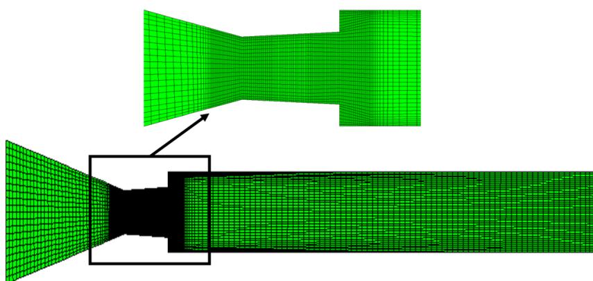
**Fig. 3.** Structural mesh for 2D planar CD nozzle for Area Ratio 2.56
