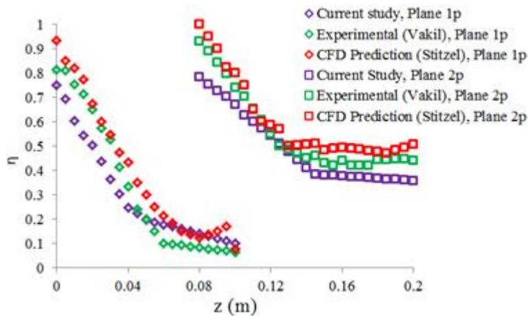
**Fig. 6.** The film cooling effectiveness comparison of planes 1p and 2p along  $y/W=0.4$
