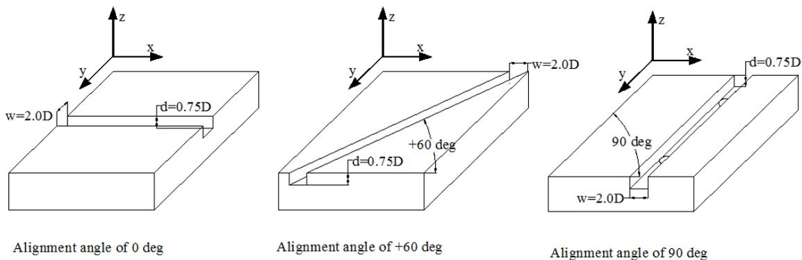
**Fig. 2.** Arrangements of row trenched cooling holes
