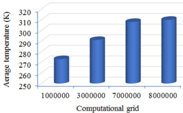
**Fig. 4.** The average temperature of all the investigated meshes in mesh independency study
