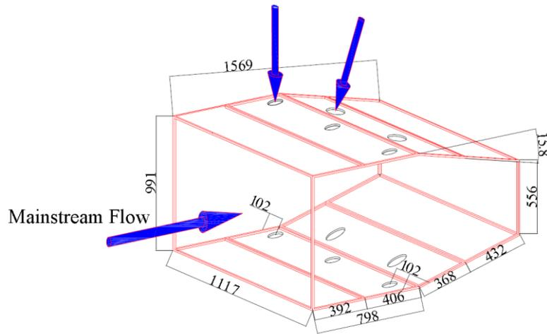
**Fig. 1.** Schematic view of the combustor simulator
