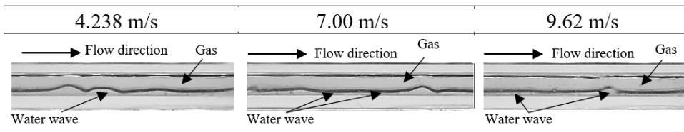
**Fig. 3.** Experimental data of Flow Pattern with  $J_L = 0.149 \text{ m/s}$  and Various of  $J_G$  with concentration of 20% glycerine
