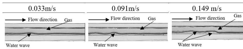
**Fig. 2.** Experimental data of Flow Pattern with  $J_G = 7.0 \text{ m/s}$  and Various of  $J_L$  with concentration of 20% glycerin
