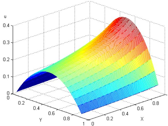
Figure 1. horizontal velocity profile for  $Kn = 0.05$
