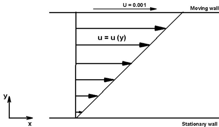
Figure 1. Geometry of a micro-couette flow.
