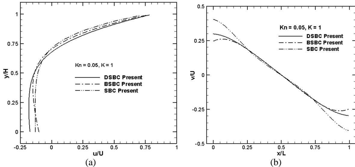
Figure 5. (a)  $u$ -velocity profile along the vertical centreline (b)  $v$ -velocity profile along the horizontal centreline for the micro-lid-driven square-cavity flow at  $Kn = 0.05$  with the BSBC, SBC and DSBC boundary conditions. Lattice size:  $300 \times 300$ .
