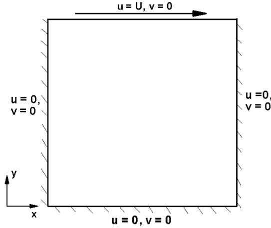
Figure 3. Geometry of a micro lid-driven cavity flow.
