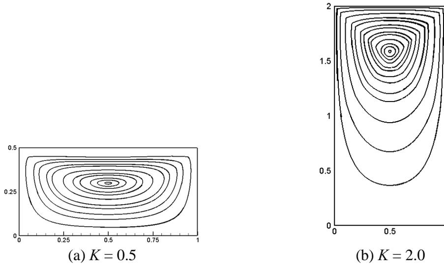
Figure 7: Streamline patterns for the micro-lid-driven cavity flow with aspect ratios  $K = 0.5$  and  $2.0$  at  $Kn = 0.10$ .
