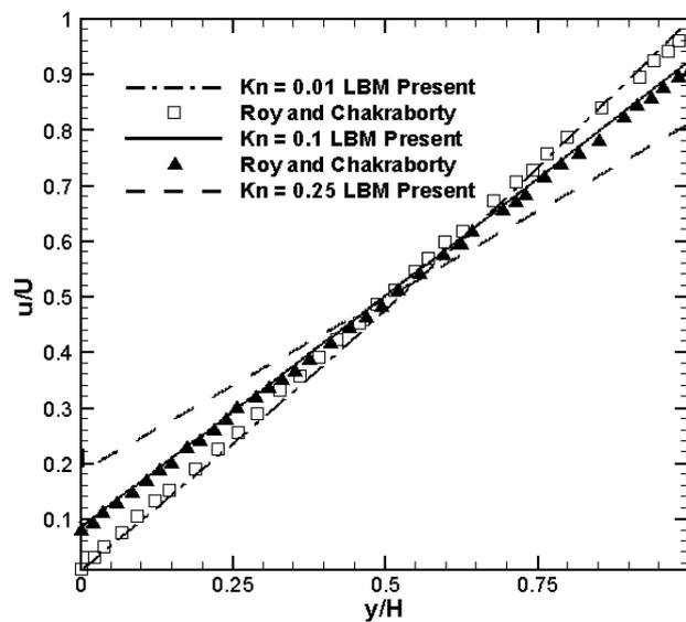
Figure 2. Micro-couette velocity profile for different  $Kn$ .
