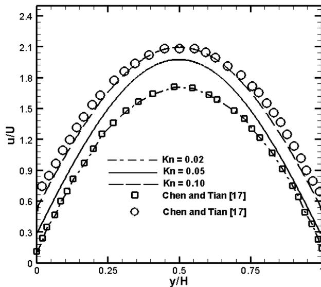
Figure 9. Velocity profiles of micro-poiseuille flow for various values of the Knudsen number.
