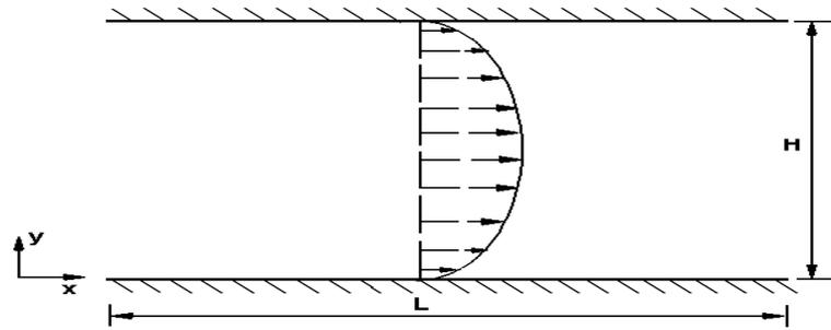
Figure 8. The geometry and micro-poiseuille flow profile.
