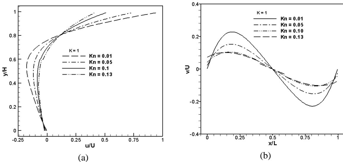
Figure 4. (a)  $u$ -velocity profile along the horizontal centreline and (b)  $v$ -velocity profile along the vertical centreline for different Knudsen numbers of the micro lid-driven square cavity flow. Lattice size:  $300 \times 300$ .
