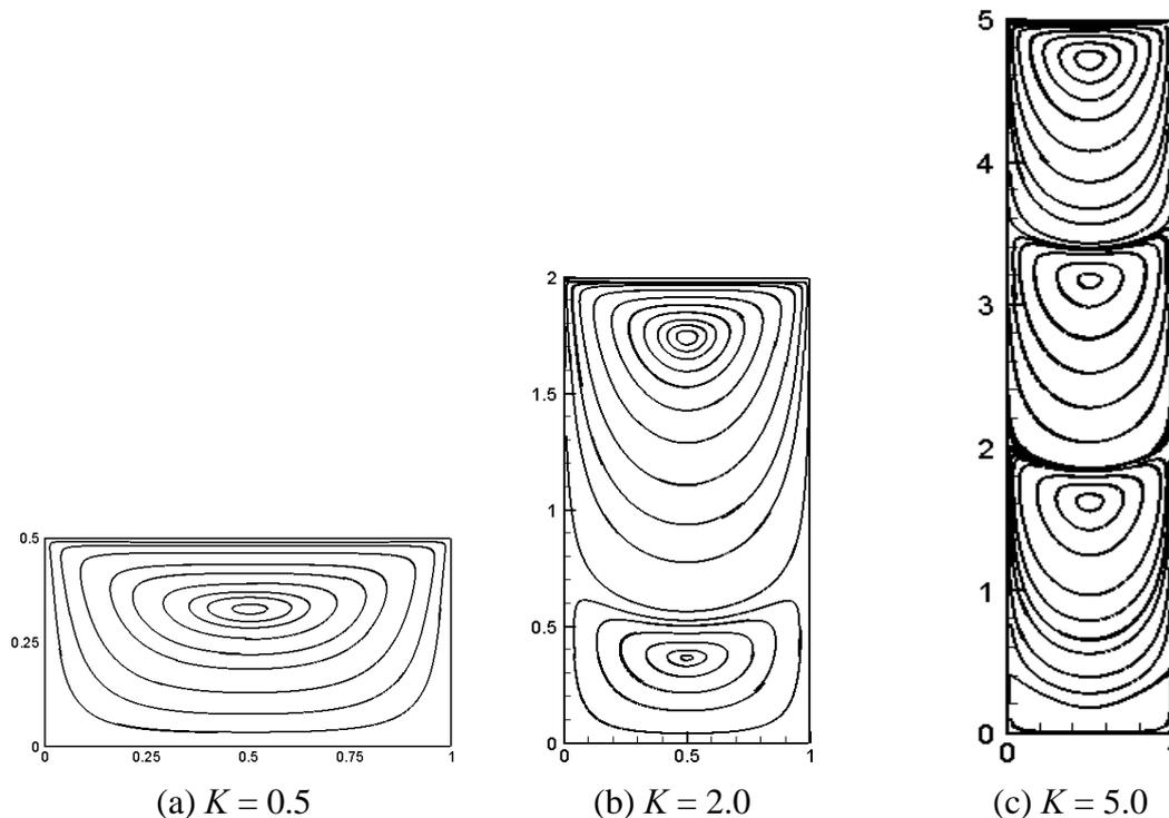
Figure 6: Streamline patterns for the micro-lid-driven cavity flow with aspect ratios  $K = 0.5, 2.0$  and  $5.0$  at  $Kn = 0.01$ .
