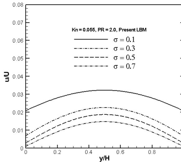
Figure 10. The effect of different TMAC on velocity profile of micro-poiseuille flow at  $Kn = 0.055$ .
