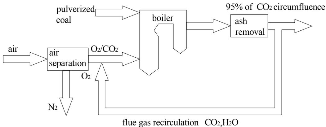
Figure 4 the schematic diagram of traditional oxygen-enriched burner
