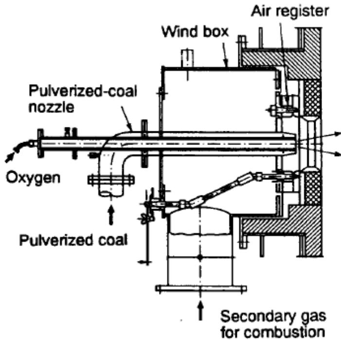
Fig.3 Oxygen-rich ignition burner
