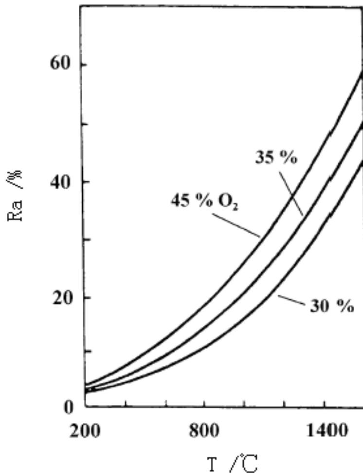
Fig 1 The relationship between smoke temperature and energy saving rate under the different oxygen concentration [8]
