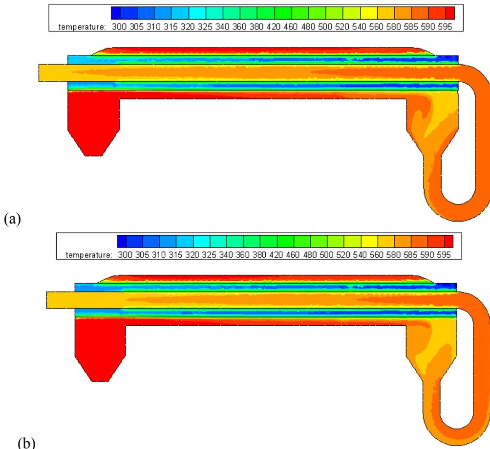
Figure 7. the temperature field under (a) the first and (b) second working conditions of the burner
