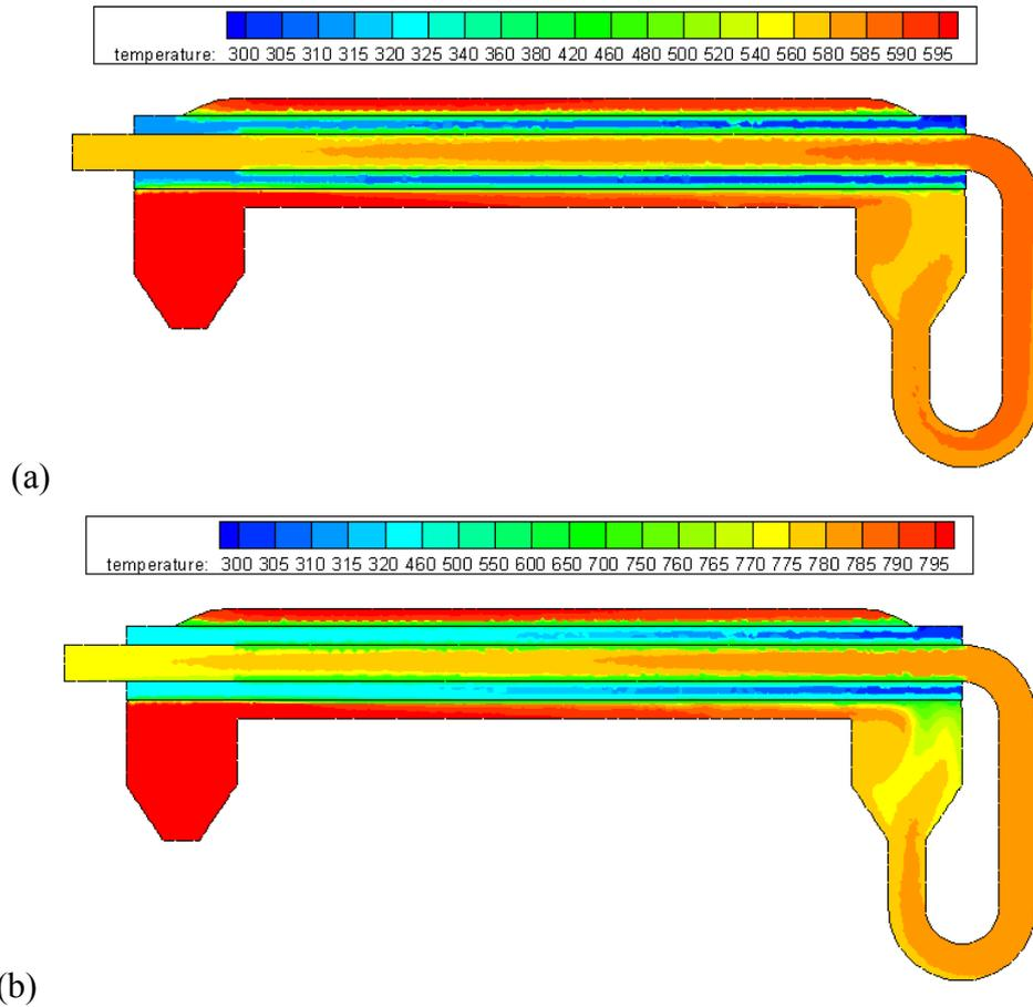
Figure 8.. The temperature field under (a) the third and (b) fourth working conditions of the burner
