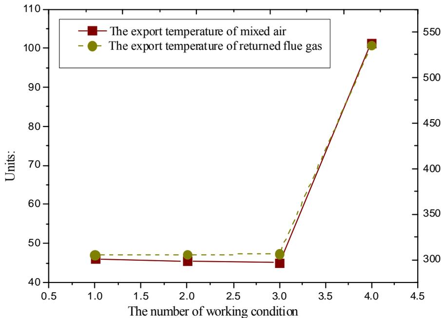
Figure 11. The export temperature of gas flow under four working conditions
