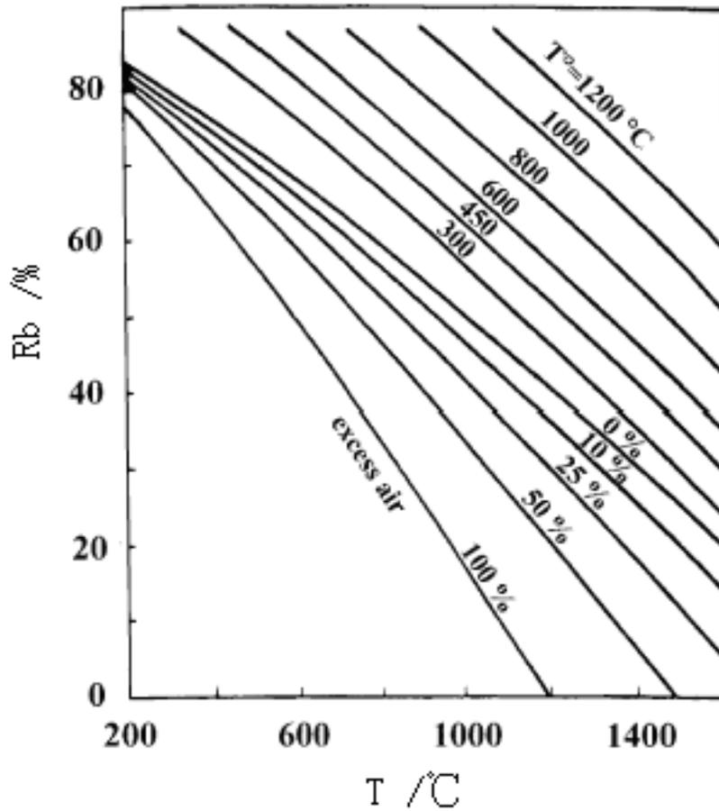
Fig 2 The relationship between unburned proportion of natural gas and exhaust temperature under the different oxygen concentration [9].
