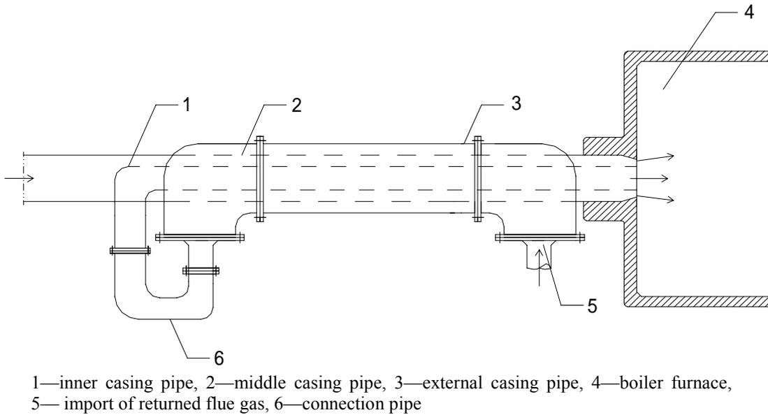
Figure 5 the schematic diagram of new type of oxygen-enriched burn
