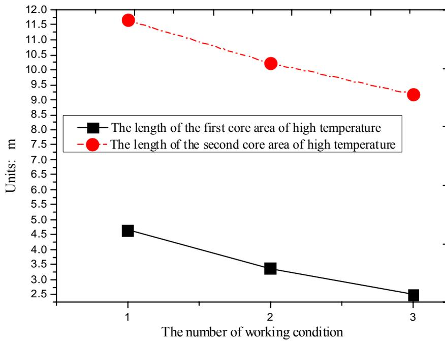
Figure 9. The length of core area of high temperature under three kinds of working condition
