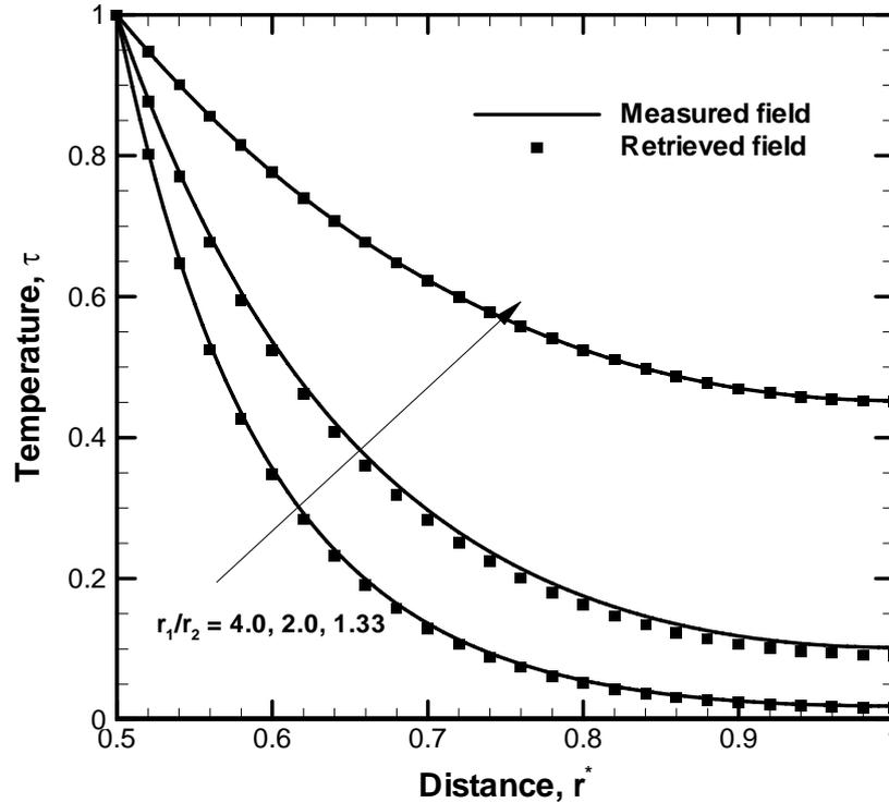
Figure 5: Comparison of the temperature fields at different locations for exact measurements and different radius-ratios;  $r_1 = 0.5\text{m}$ ,  $r_2 = 1.0\text{m}$ ,  $h = 150\text{W}/\text{m}^2\text{K}$ ,  $K = 200\text{W}/\text{mK}$ .
