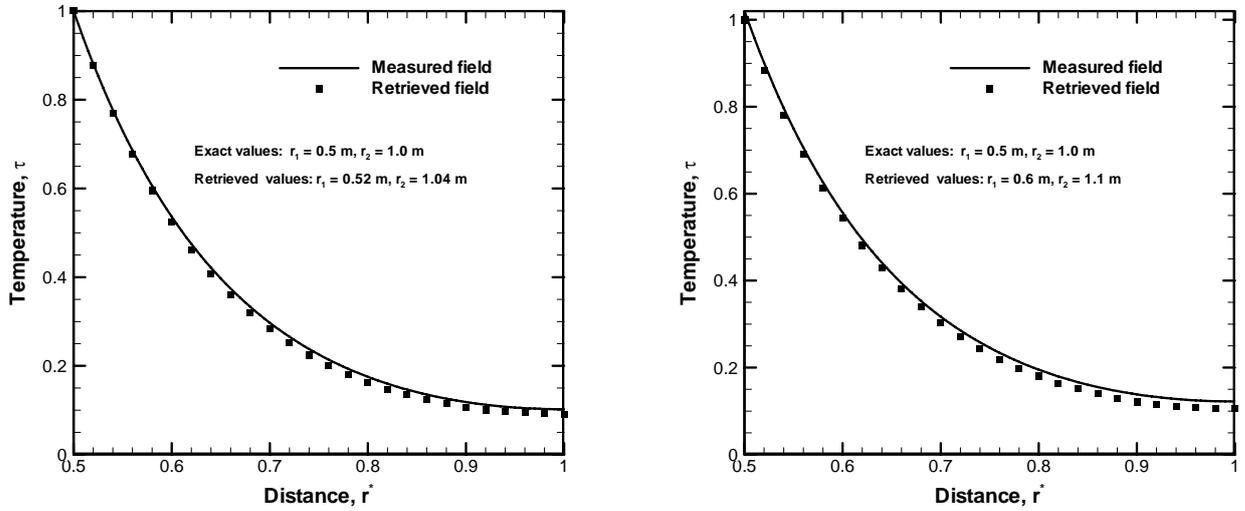
Figure 4: Comparison of local temperature fields at different locations; (a) exact temperature measurements; (b) temperature measurements with measurement error
