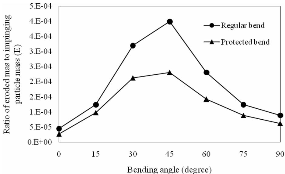
Figure 5. Comparison of eroded mass with respect of impinging particle mass for both regular and protected bends in different bending angles.
