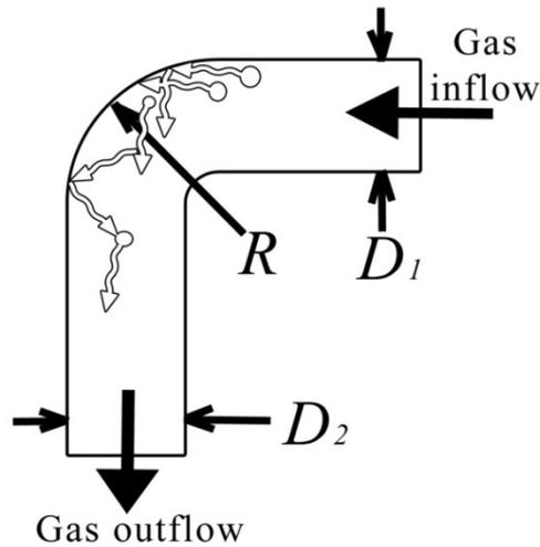
Figure 1. Schematic of gas-particle flow transpots through the bend
