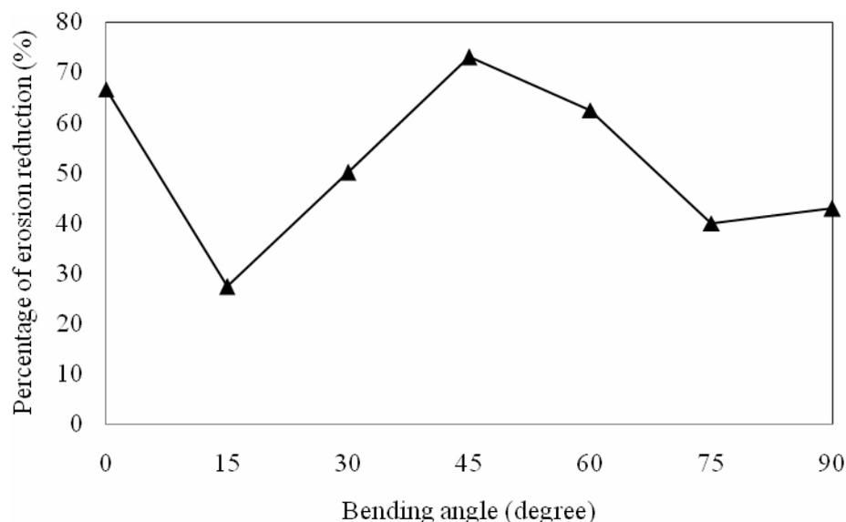
Figure 6. Erosion reduction for protected bend with respect to regular bend in different bending angles.
