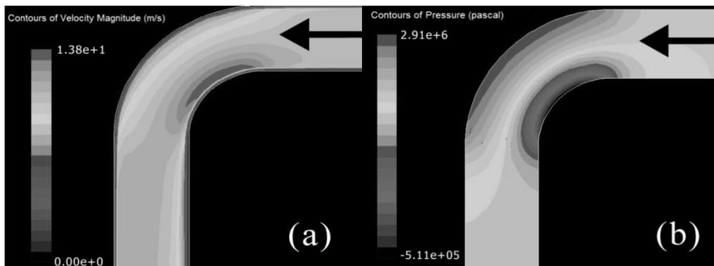
Figure 2. Contours of velocity(a) and pressure(b) inside of the regular bend
