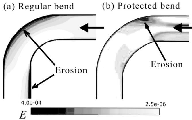
Figure 4. Contours of eroded mass parameter for both regular and protected bends
