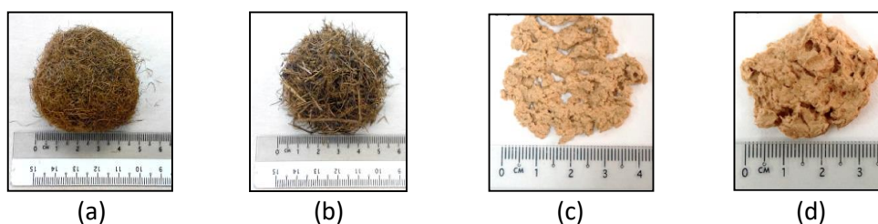
Fig. 1. Macro photographs of (a) as-received FSTL, (b) as-received CSTL, (c) fibrillated FSTL and (d) fibrillated CSTL fibers
