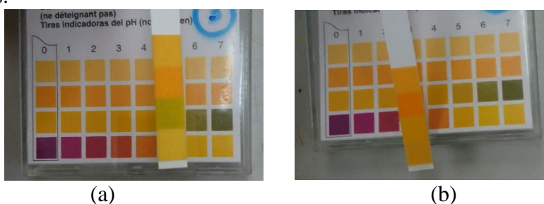
Fig. 1. The pH value of OPE extracted using (a) Ethanol (pH = 6); (b) Distilled water (pH = 5)
