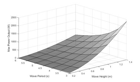
Fig. 9. Maximum power output of point absorber for configuration EI under different wave heights and wave periods
