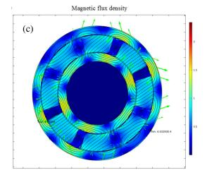
Fig. 4. Magnetic flux density for configurations (a) EX, (b) IN, and (c) EI
