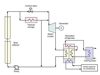
Fig. 2. Schematic diagram of solar thermal cogeneration system
