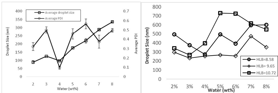
**Fig. 2.** Droplet size of nano-emulsions as a function of water percentage (wt%). Surfactant wt% was fixed at 6 wt%
