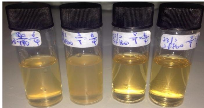
**Fig 4.** Water-in-diesel nano-emulsion at varying water wt%, i.e. 5 wt%, 4 wt%, 3 wt% and 2 wt% from the left
