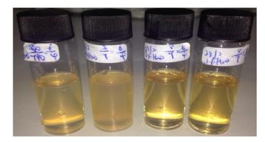
Fig 4. Water-in-diesel nano-emulsion at varying water wt%, i.e. 5 wt%, 4 wt%, 3 wt% and 2 wt% from the left
