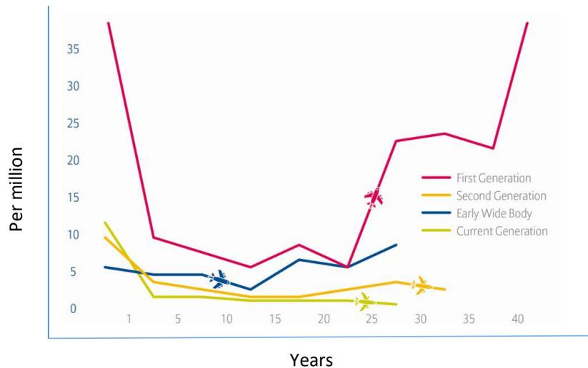
Fig. 5. Accident Rates Jet Aircraft by Generation per 1 million departures [50]
