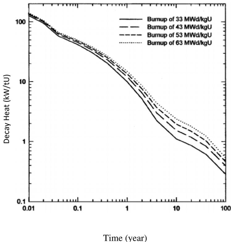
Fig. 2. Decay heat as a function of time from 0.1 years to 100 years
