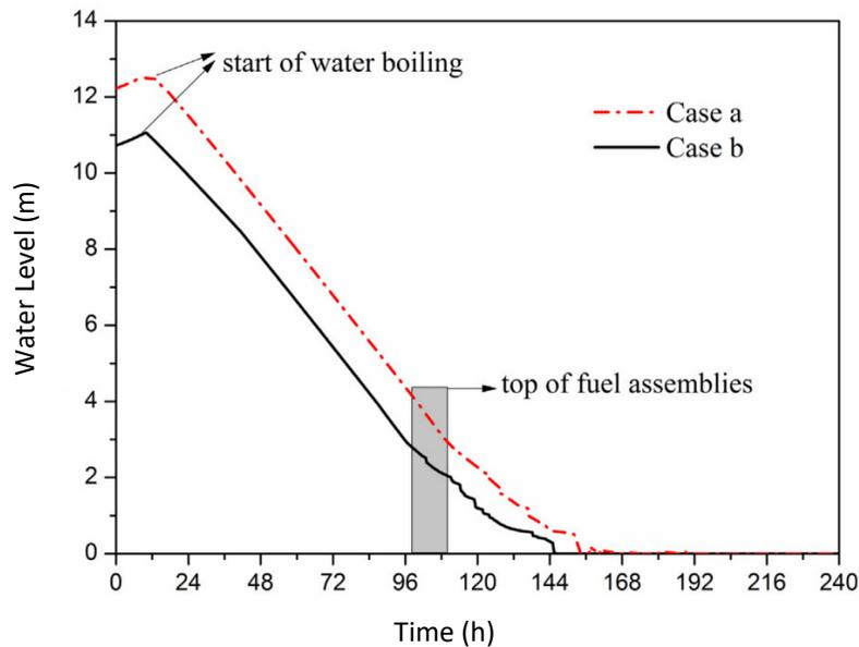
**Fig. 4.** Water level in SFP under the condition of different initial water levels
