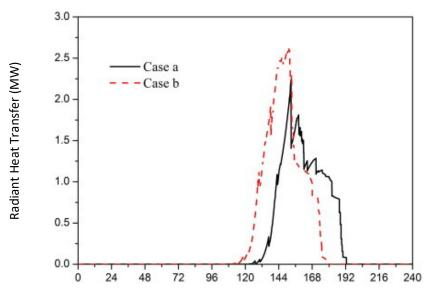
Time (h) **Fig. 1.** Analysis of the loss of pool cooling accident in a PWR spent fuel pool with MAAP5 [26]
