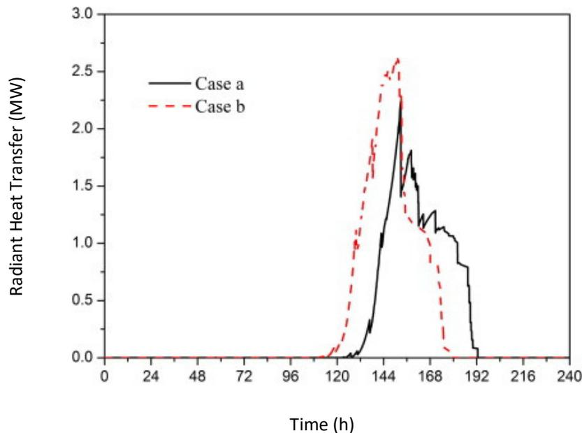
**Fig. 1.** Analysis of the loss of pool cooling accident in a PWR spent fuel pool with MAAP5 [26]
