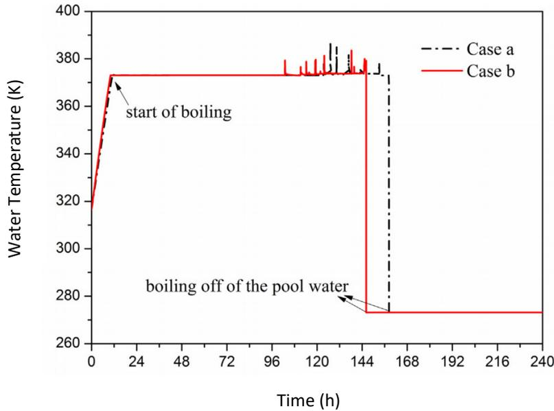
**Fig. 3.** Water temperature in SFP under the condition of different initial water levels
