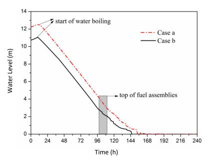
Fig. 4. Water level in SFP under the condition of different initial water levels
