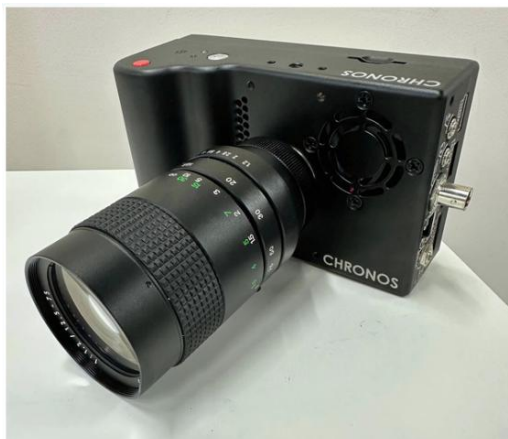
Fig. 6. High speed camera utilized to capture detailed flow behaviour at the pump section
