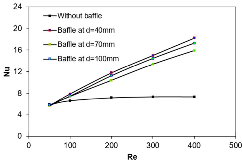
**Fig. 6.** Average Nusselt number of the channel with and without baffle
