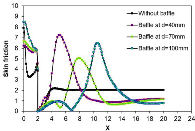
**Fig. 7.** Local skin friction of the channel with and without baffle at  $Re=200$
