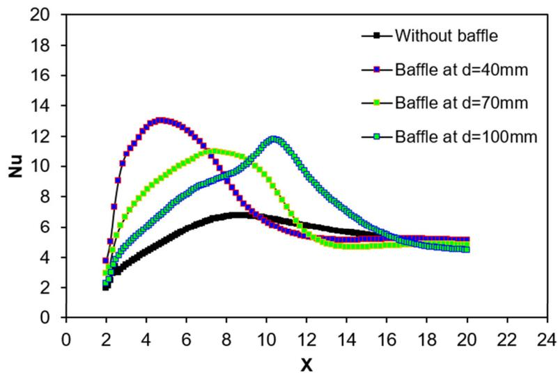
**Fig. 5.** Local Nusselt number of the channel with and without baffle at Re=200
