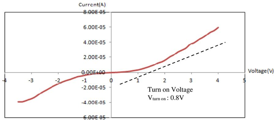
**Figure 2 :** Current-voltage (I-V) characteristics of Au/n-ZnO/p-TIPS-pentacene/ITO/plastic Schottky barrier diode
