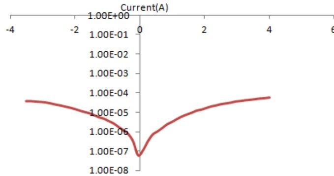
**Figure 3 :** Semi-logarithmic I-V characteristics of Au/n-ZnO/p-TIPS-pentacene/ITO/plastic Schottky barrier diode
