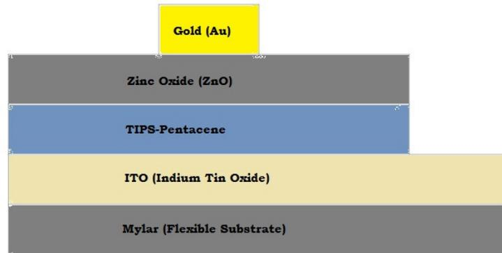
**Figure 1:** Organic diode architecture on flexible substrate
