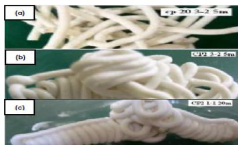
**Fig. 2.** Moldable form of CPC after injection: CP20 (3:2) after 5min (a); CP2 (3:2) after 5 min (b); CP2 (1:1) after 20min (c) [30].
