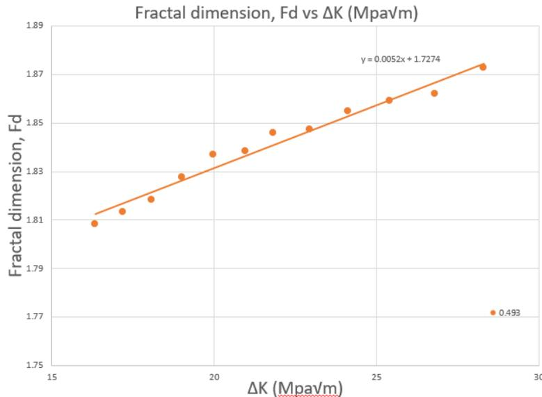
**Fig. 4.** Relationship between Stress Intensity Factor and Fractal Cracks Propagation in AISI 410 Steel
