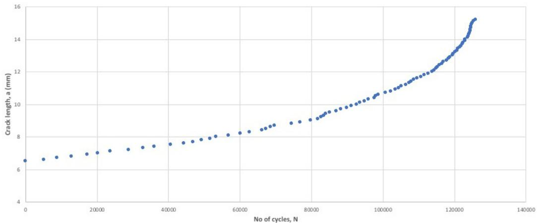
**Fig. 1.** Fatigue Crack Growth Behavior Test – AISI 410
