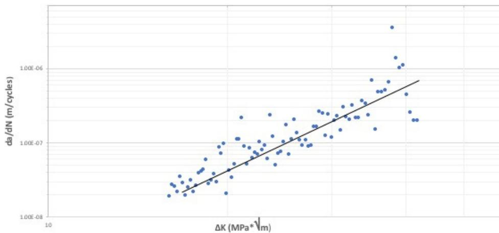
**Fig.2.** Relationships between stress intensity factor range  $\Delta K$  and crack growth rate  $da/dN$
