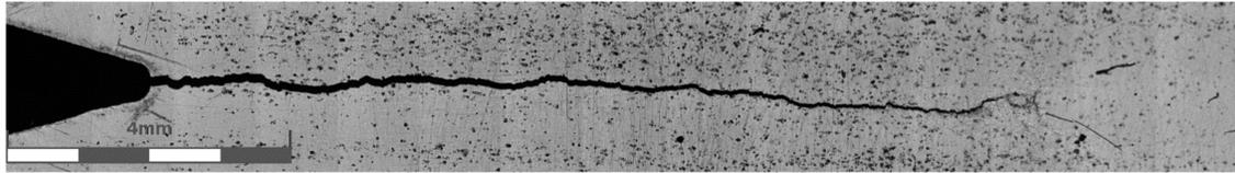
**Fig. 3.** Crack propagation under 100x digital microscope
