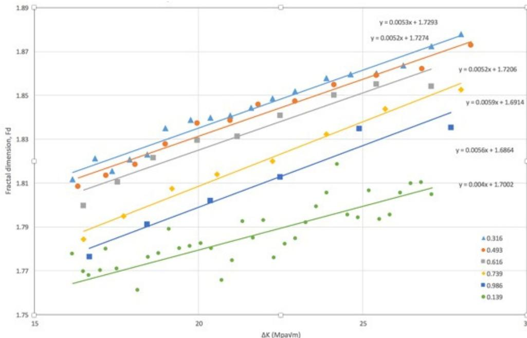
**Fig. 4.** Comparison between different window sizes for  $F_D$  and  $\Delta K$
