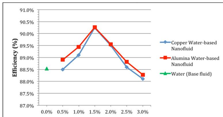
**Figure 8:** Efficiency of domestic water heat exchanger.
