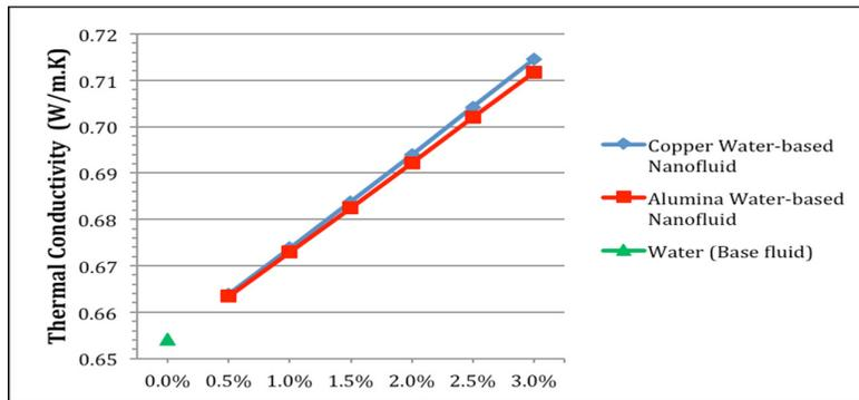
**Figure 6:** Thermal conductivity of heat transfer fluids.
