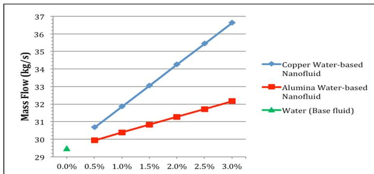
**Figure 7:** Mass flow of heat transfer fluids.
