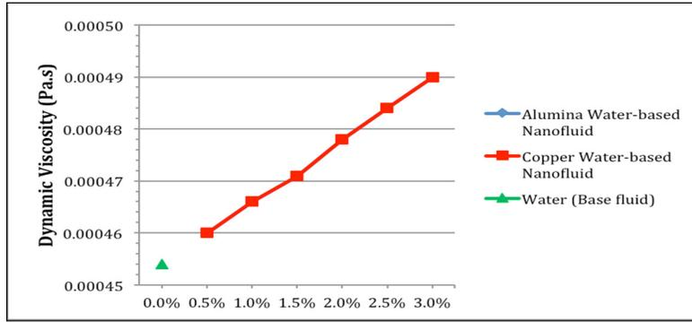
**Figure 5:** Dynamic viscosity of heat transfer fluids.
