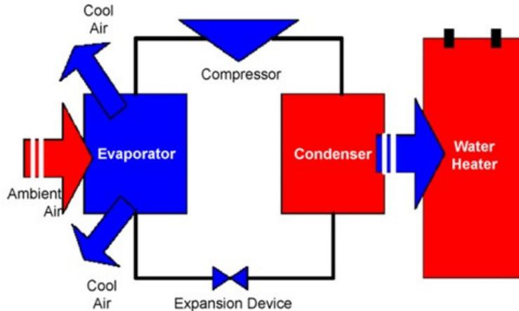
**Figure 1:** A schematic of domestic water heating system [1].
