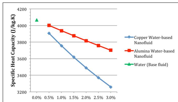
**Figure 4:** Specific heat capacity of heat transfer fluids.
