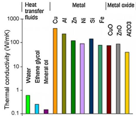
**Figure 2:** Comparison of the thermal conductivity of common heat transfer liquids and solids of metal and metal oxide. [15]
