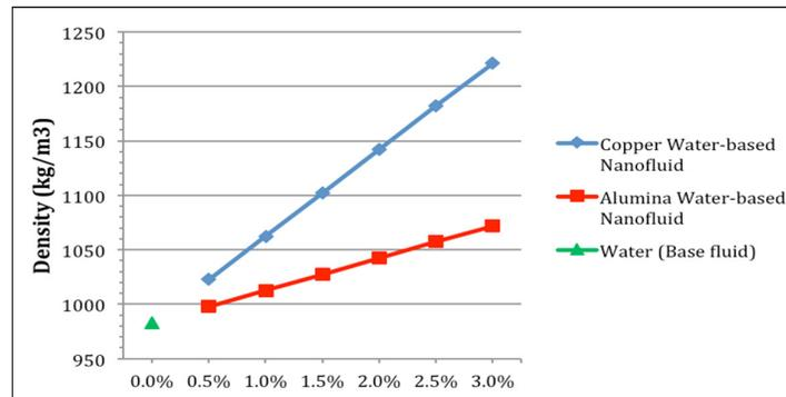
**Figure 3:** Density of heat transfer fluids
