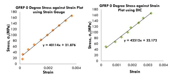
Figure 15: Stress against Strain Plot for GFRP 0 Degree Unidirectional Tensile Test
