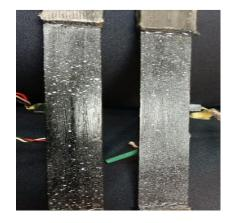
Figure 4: Speckle pattern obtained from black/white paint using air spray
