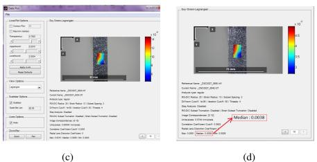
**Figure 14:** (a)Strain Exx contour, (b) Strain Eyy Contour, (c) Strain Exy contour and (d) Strain Exy contour and median value
