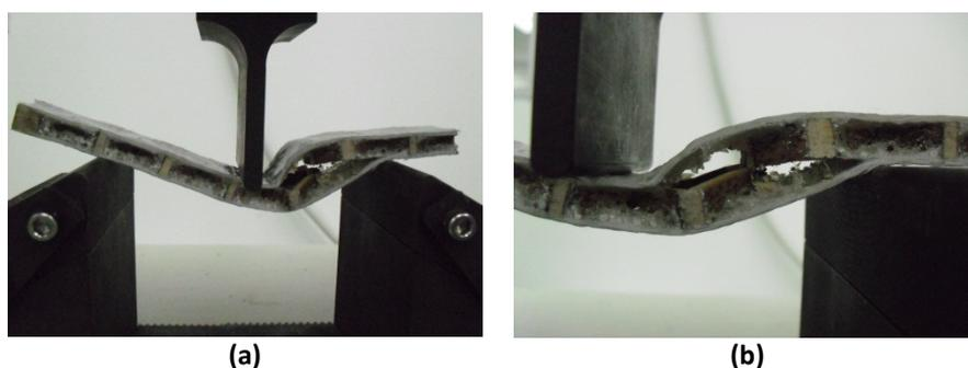
Fig. 4. Failure of core and glass fiber facesheet
