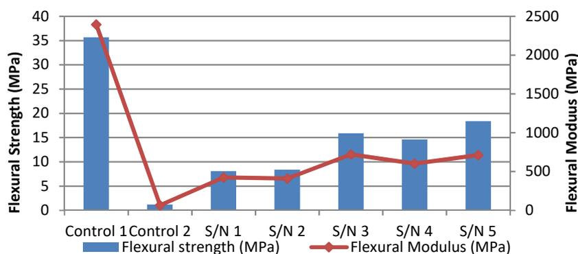
**Fig. 2.** Flexural strength and flexural modulus versus different composites
