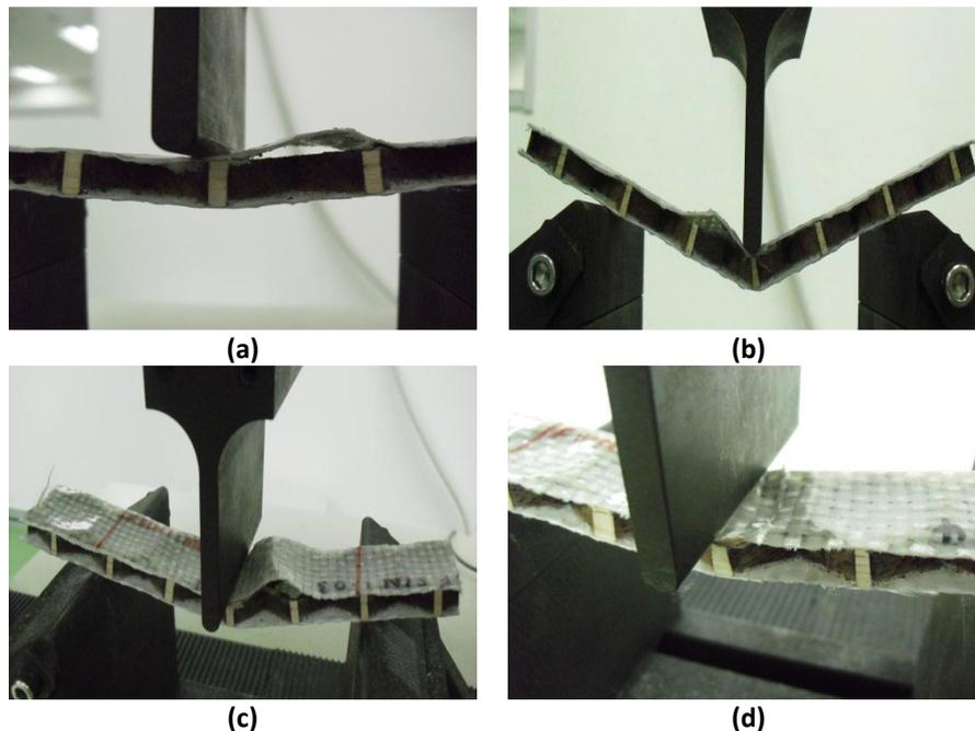
Fig. 5. Delamination at the top facesheet of specimen
