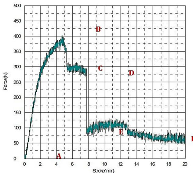
Fig. 3. Force-stroke curve for SN 1-6 for flexural test
