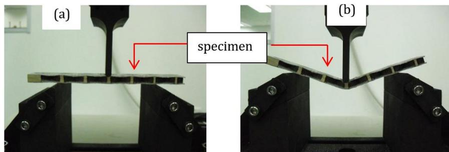
**Fig. 1.** Flexural test (a) beginning of test (b) ending of test
