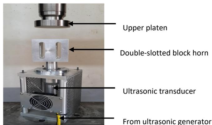
**Fig. 4.** Ultrasonic compression test set-up
