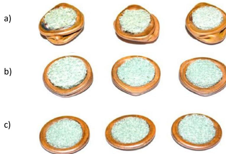
**Fig. 6.** Deformation profile of copper tube filled with PVC closed-cell foam for (a) quasi-static, (b) intermittent ultrasonic and (c) continuous ultrasonic compression test
