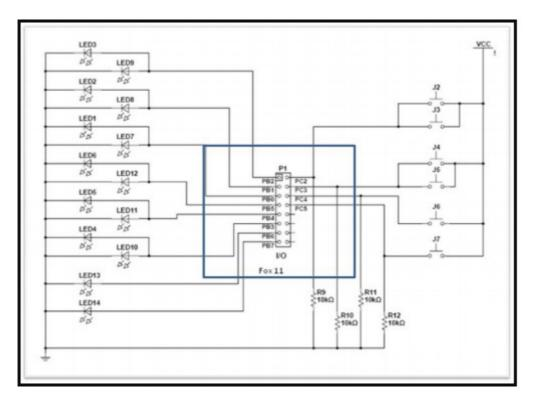
Fig. 6. Circuit Diagram of the Intelligent Traffic Control
