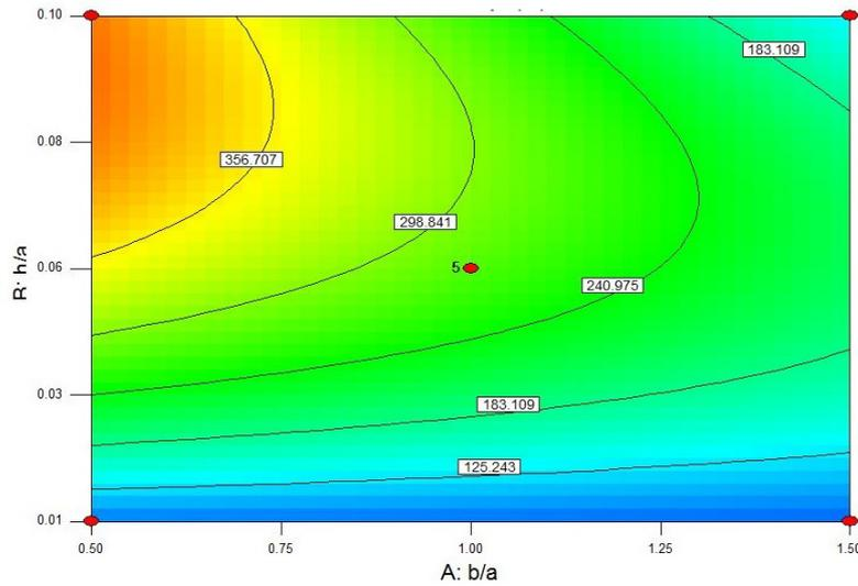
**Fig. 5.** Contour plot of fundamental frequency (thickness ratio vs. aspect ratio)
