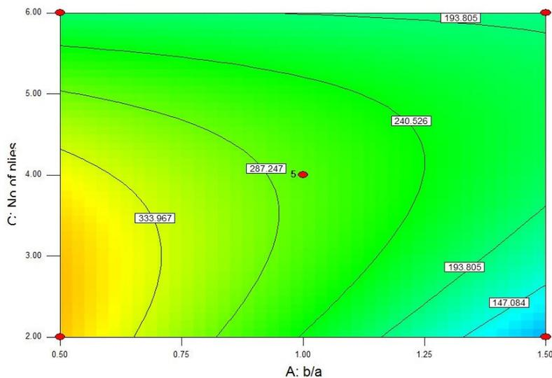
**Fig. 6.** Contour plot of fundamental frequency No. of plies vs. aspect ratio)
