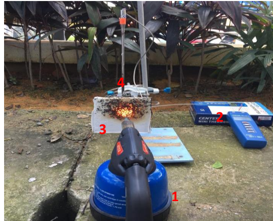
Fig. 2. Bunsen burner test setup (1) Bunsen burner, (2) digital thermometer, (3) sample and (4) thermocouple plate
