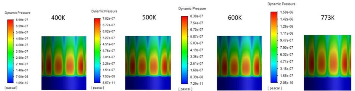
**Fig. 7.** Dynamic pressure distribution in cold volume of the cylinder engine for every temperature
