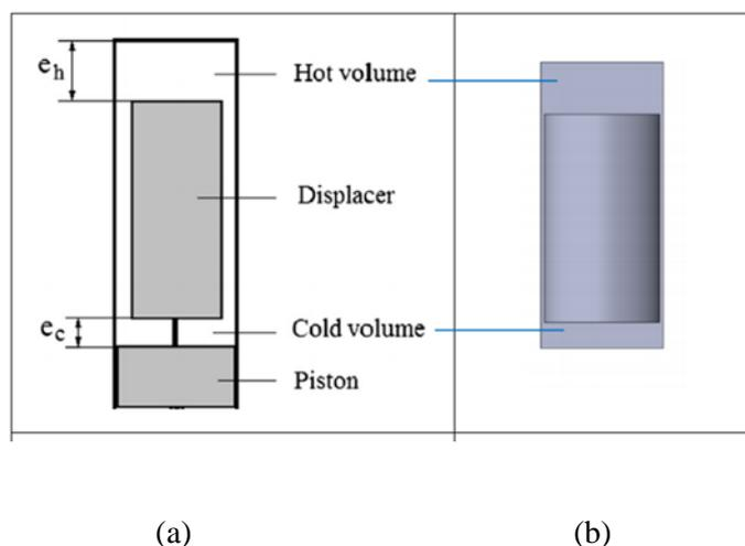
Fig. 2. (a) Schematic diagram and (b) CFD Domain
