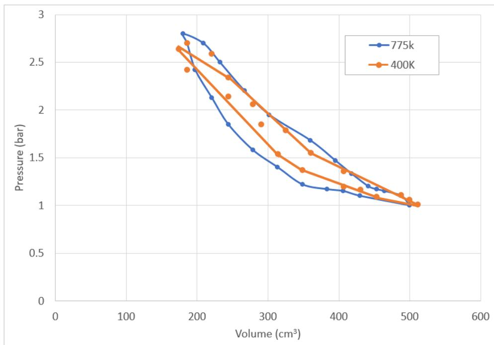
**Fig. 8.** Volume and Pressure relation between heat source temperature 400K and 775K
