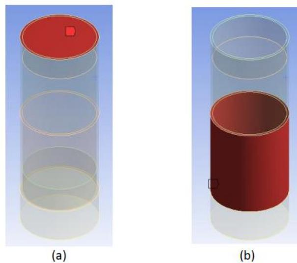
**Fig. 5.** Two boundary condition for heat source (a) hot surface and (b) cold source surface
