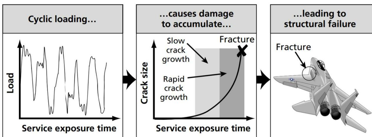
Fig. 1. Fatigue Cracks under cyclic loading and structural failure
