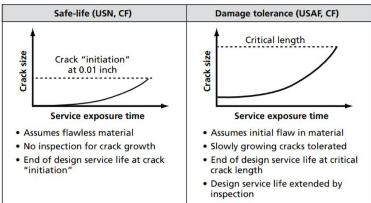
**Fig. 2.** Comparison of Safe-Life and Damage Tolerance
