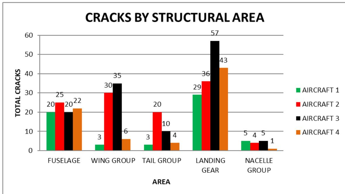
**Fig. 6.** Cracks by Structural Area
