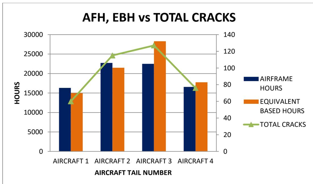
**Fig. 7. Airframe Hours, EBH, and Total Cracks**
