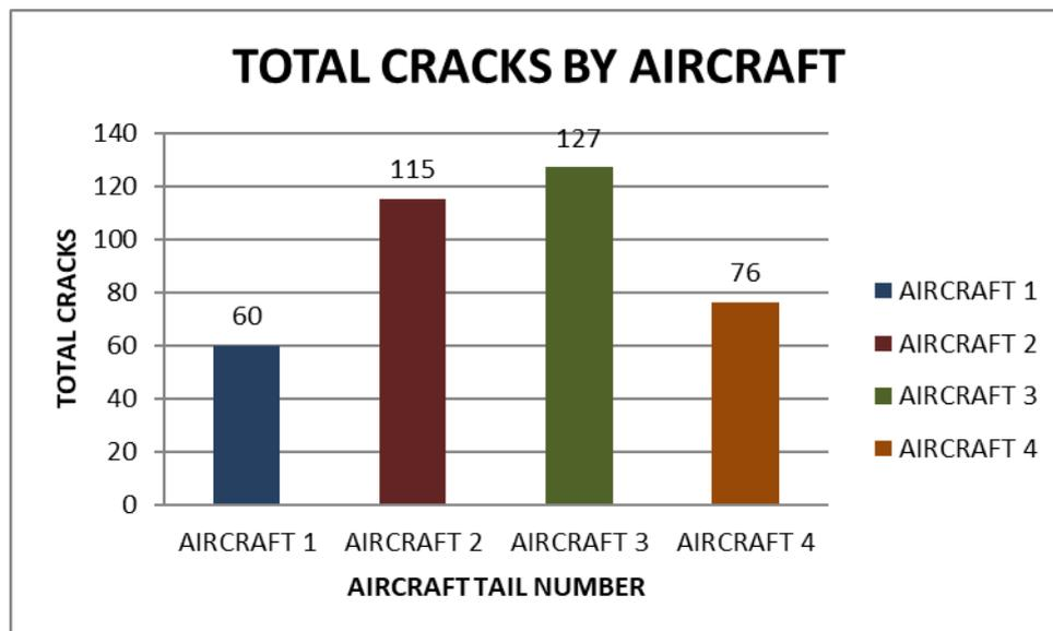
**Fig. 5.** Total Crack Occurrences from year 1994 to 2018
