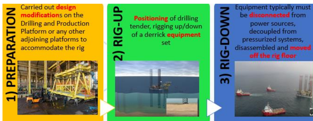
Fig. 2. Infill drilling stages in BYDP-B platform
