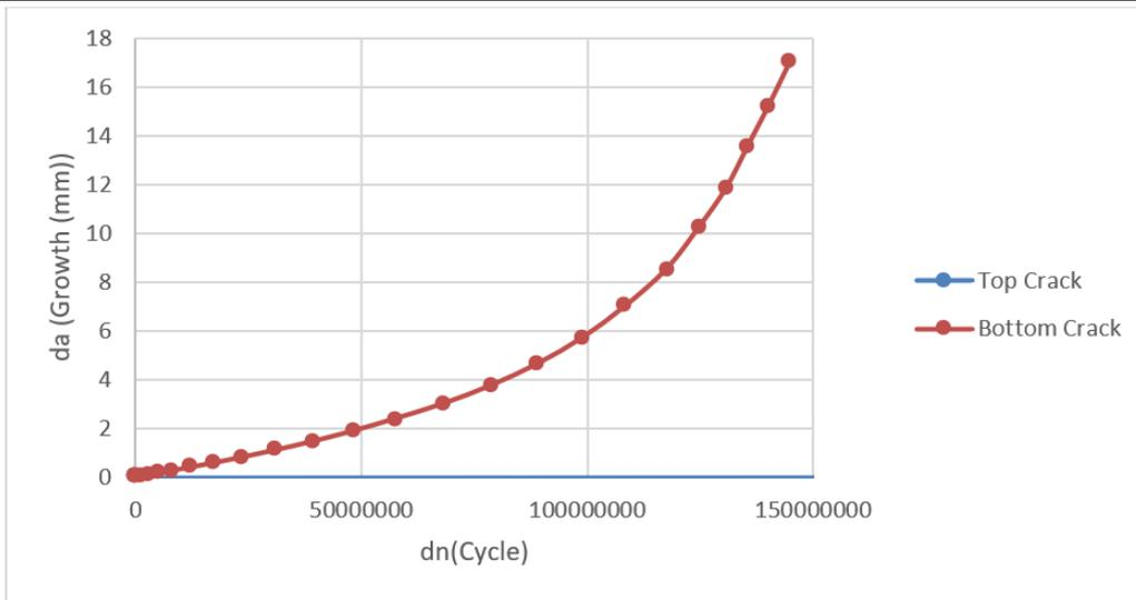
**Fig. 10.**  $dn$  vs  $da$  for top and bottom crack
