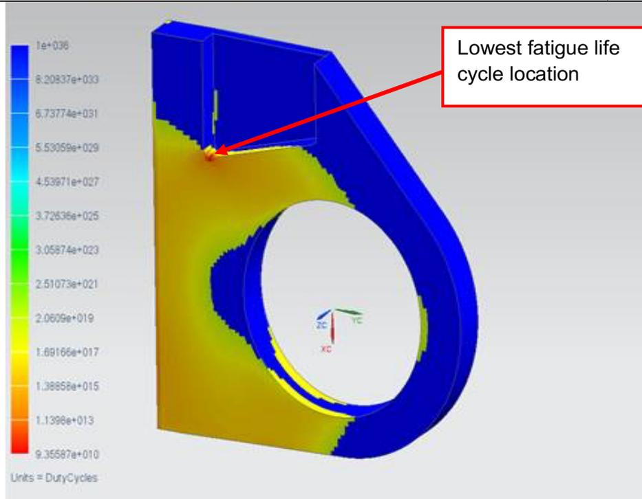
Figure 17. Fatigue Life Cycle Result
