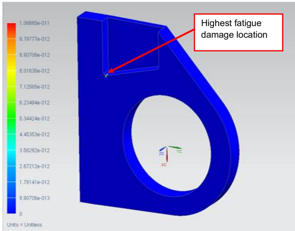
**Fig. 16.** Fatigue Damage Result
