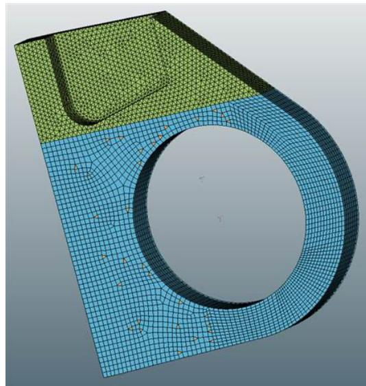
Fig. 5. ZENCRACK horizontal stabiliser lug structure part model
