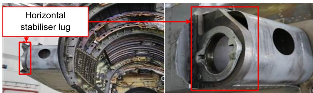
Fig. 1. Location of the horizontal stabilizer lug
