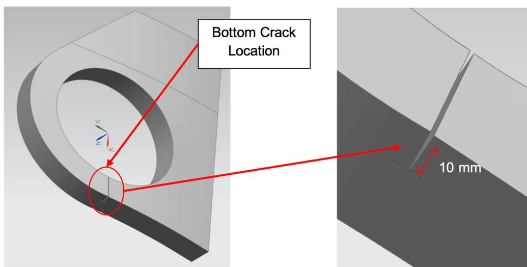
Fig. 6. Bottom crack location on the horizontal stabilizer lug structure part model
