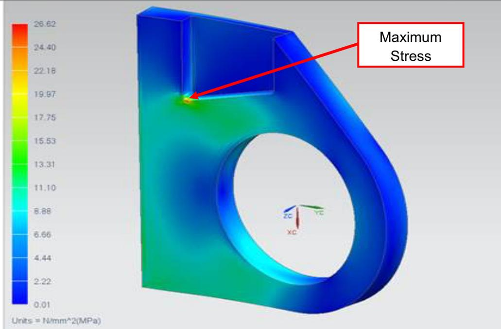
**Fig. 14.** Stress result of the analysis part
