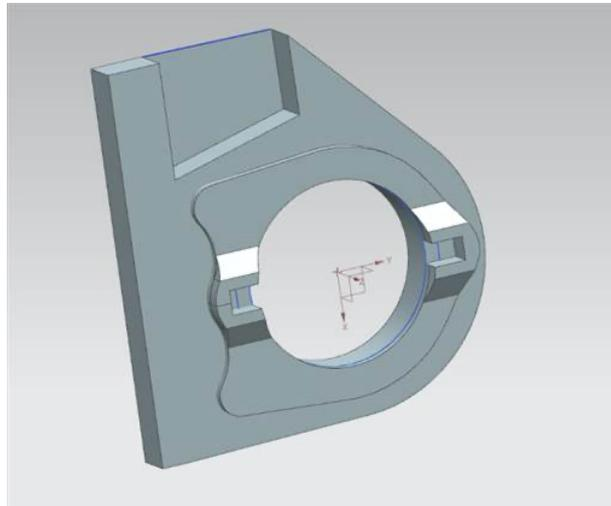
**Fig. 2.** Obtained horizontal stabiliser lug model
