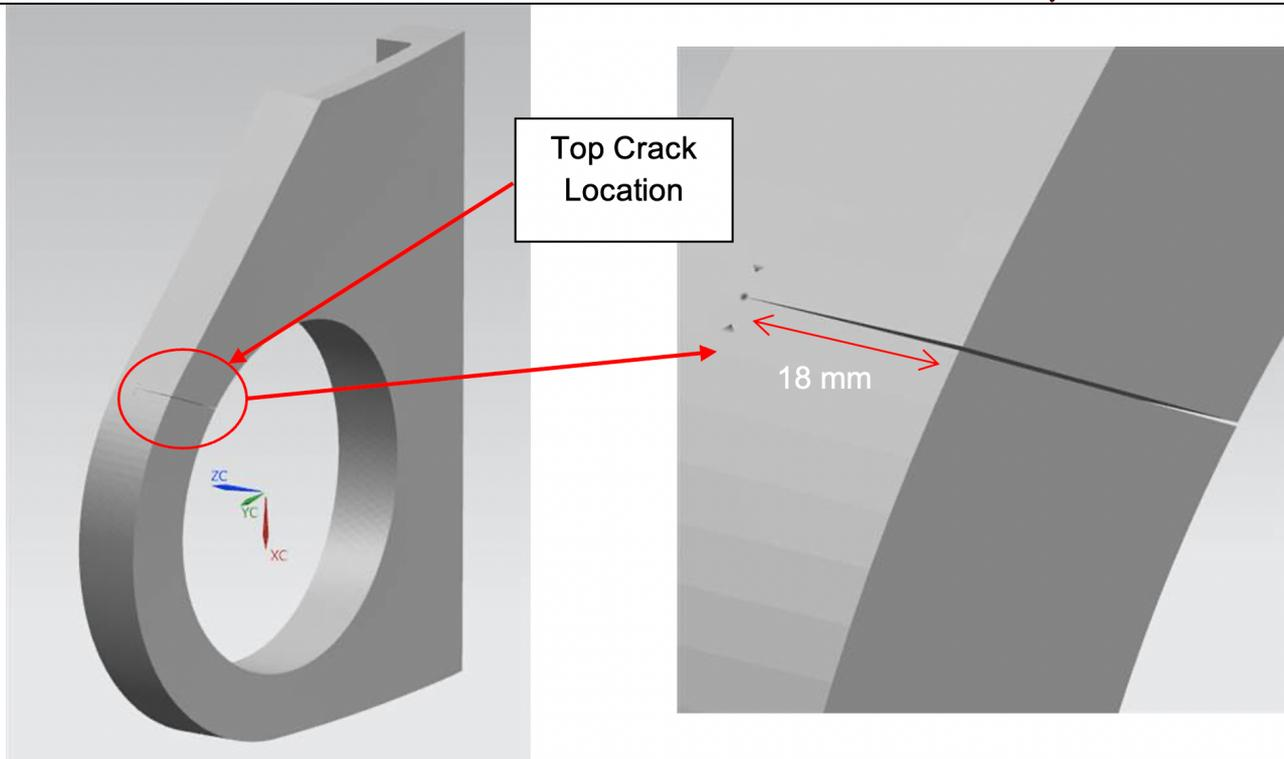
**Fig. 7.** Top crack location on the horizontal stabilizer lug structure part model
