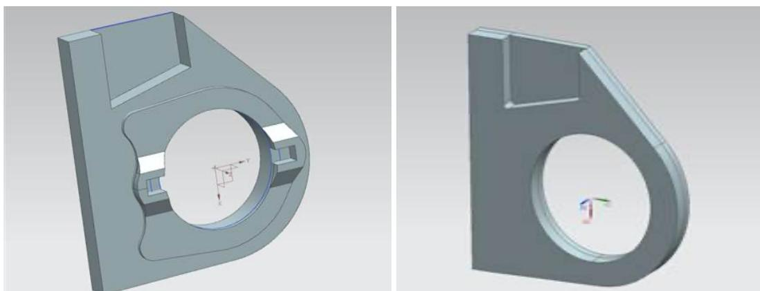
**Fig. 8.** Scanned horizontal stabilizer lug (left) and after clean-up process (right)
