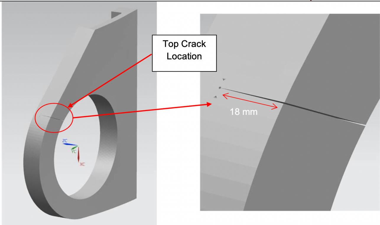
**Fig. 7.** Top crack location on the horizontal stabilizer lug structure part model
