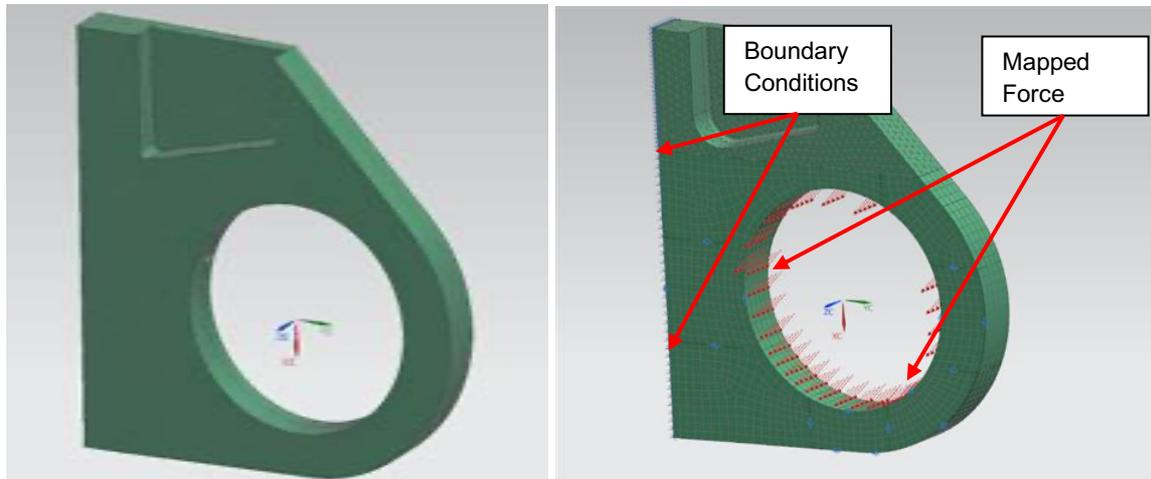
**Fig. 9.** Mesh model (left) and mapped loading on the horizontal stabilizer lug model (right)
