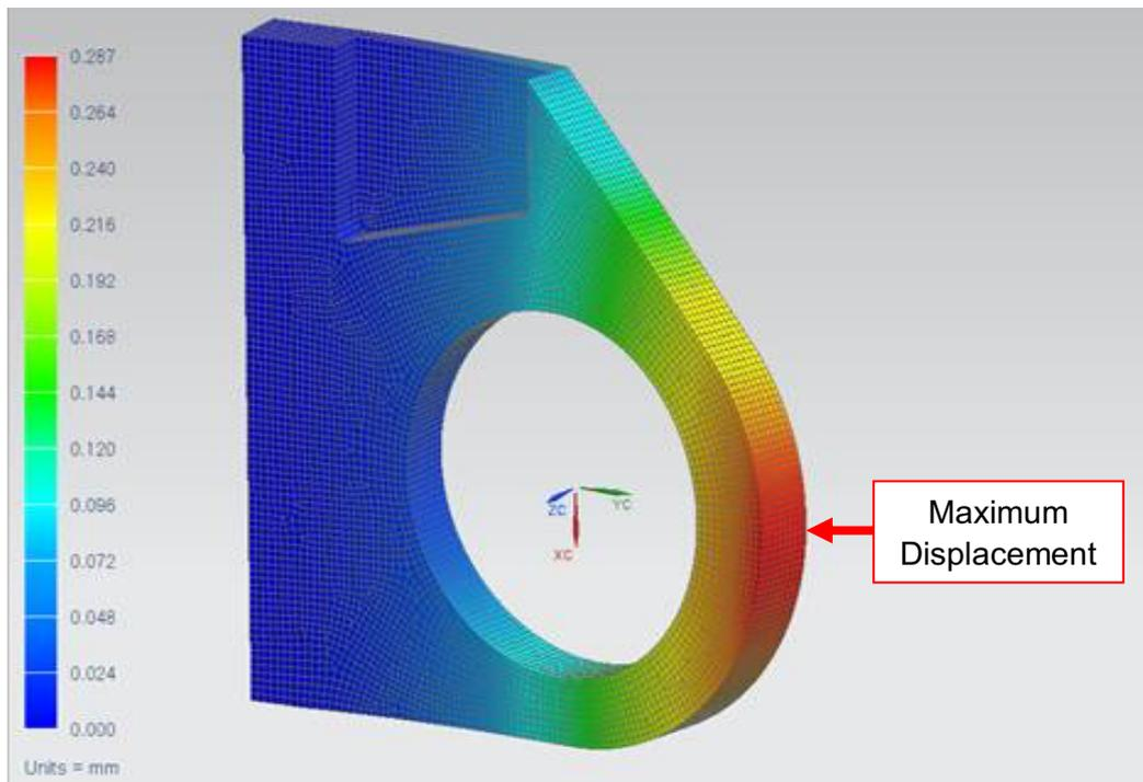
**Fig. 13.** Displacement result of the analysis part
