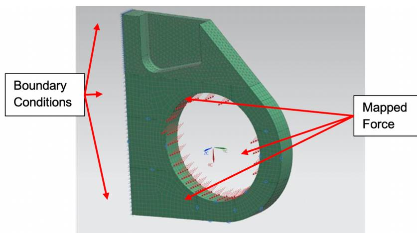
**Fig. 4.** Mapped loading on the horizontal stabilizer lug structure part model
