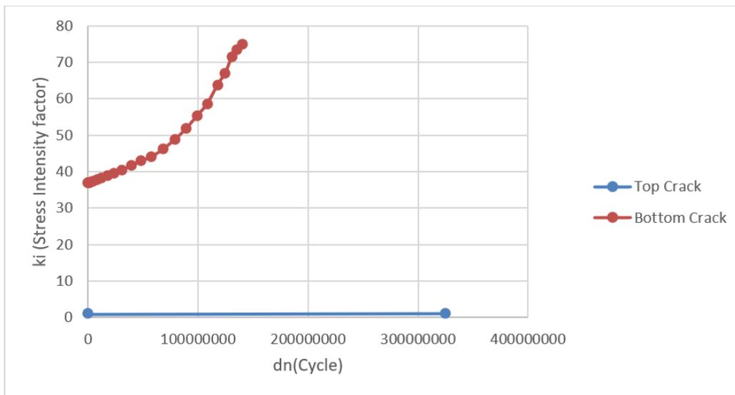
**Fig. 11.**  $dn$  vs  $k_i$  for top and bottom crack
