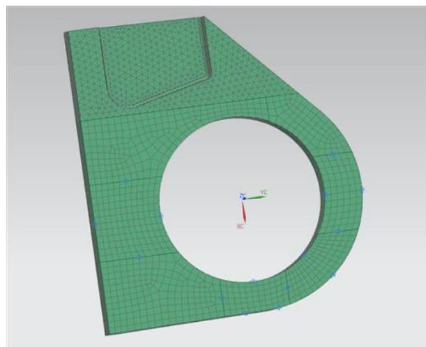
**Fig. 3.** Obtained horizontal stabiliser lug mesh model.
