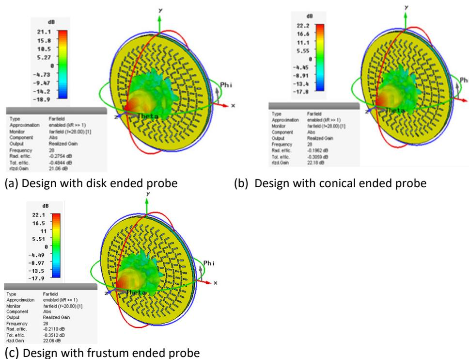
Fig. 4. 3D simulated radiation pattern
