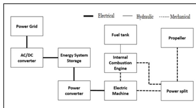
**Fig. 3.** Schematic illustration of PHERB powertrain [19]
