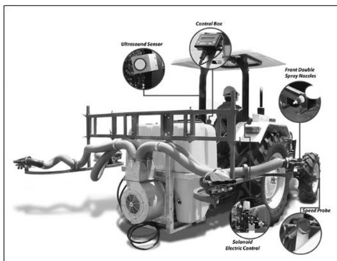
**Fig. 3.** A tractor sensor-based spraying system
