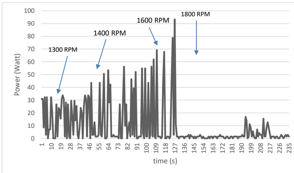
Fig. 10. Power at various engine speed
