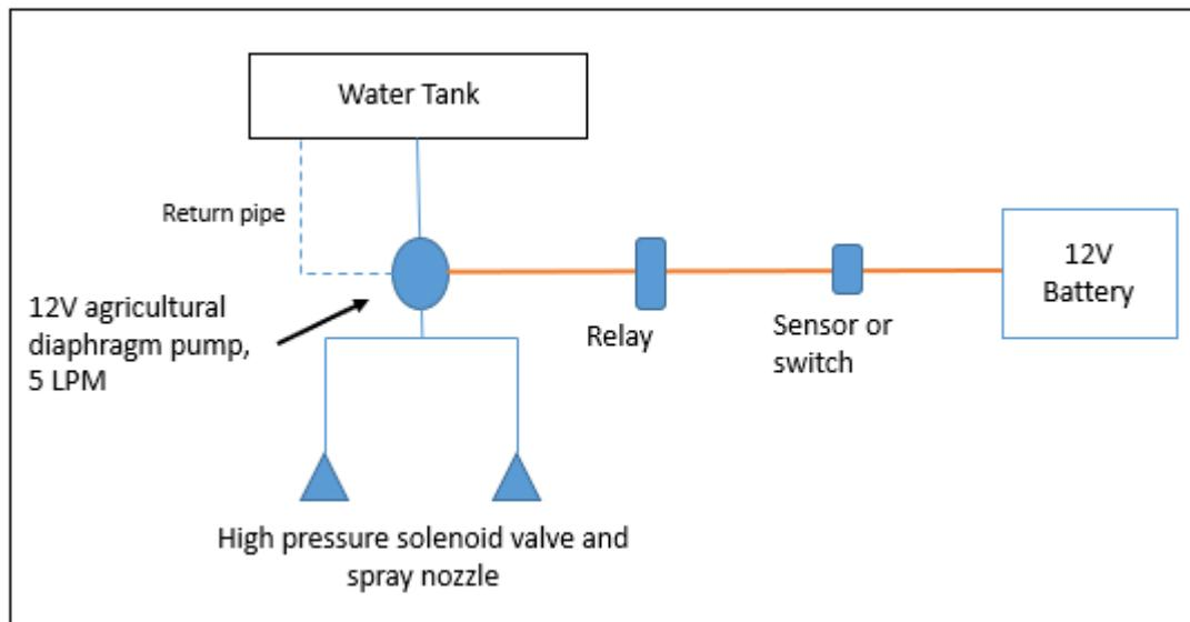
**Fig. 2.** Schematic diagram of the proposed spraying system
