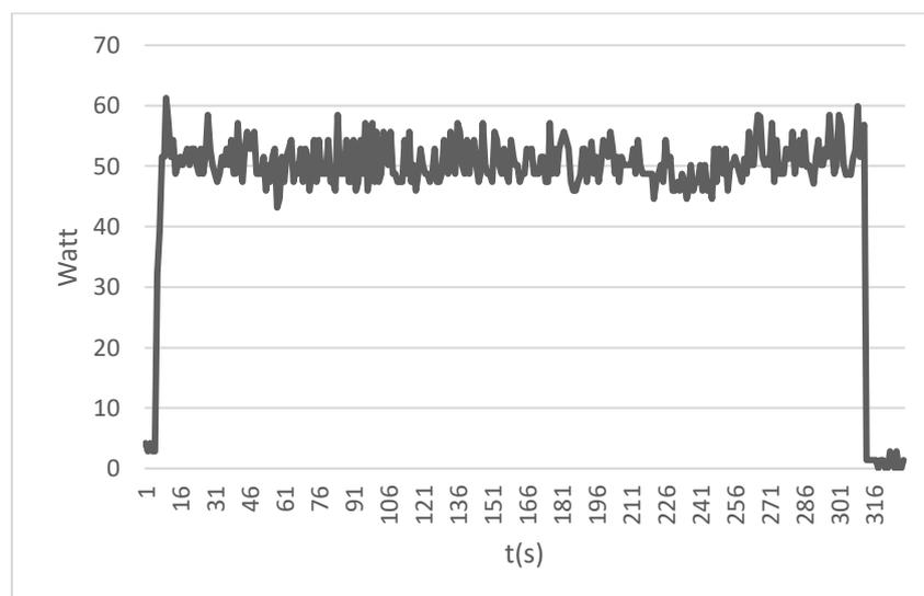
**Fig. 9.** Power consumption of the electric pump at the flow rate of 2.3 l/m
