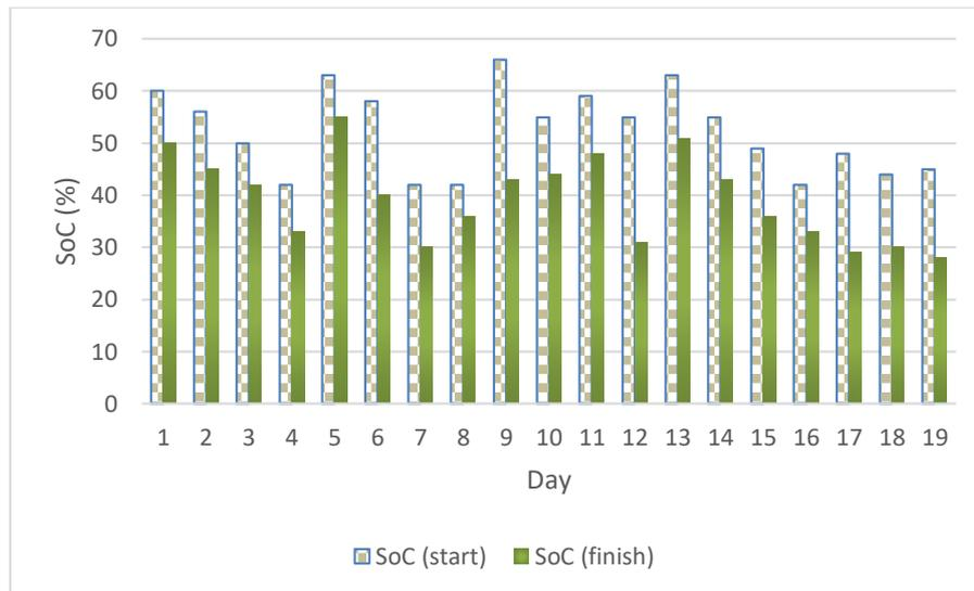
**Fig. 13.** Battery State of Charge (SOC) before and after work conducted during the field trial
