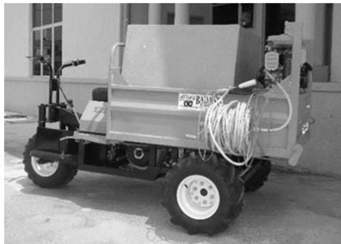
**Fig. 2.** A conventional 3-wheel type vehicle used in oil palm plantations for weedicide operation
