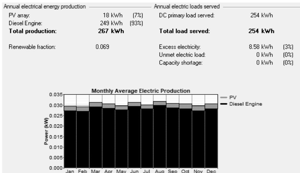
**Fig. 6.** HOMER analysis result of the rectifier generator and 10 W solar panel for the agro-hybrid application
