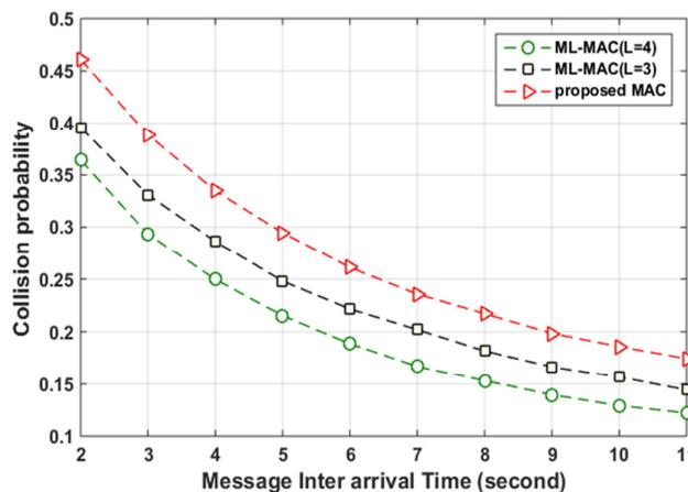
**Fig. 13.** Probability of collision for the ML-MAC (L=3&L=4) and the proposed MAC protocols
