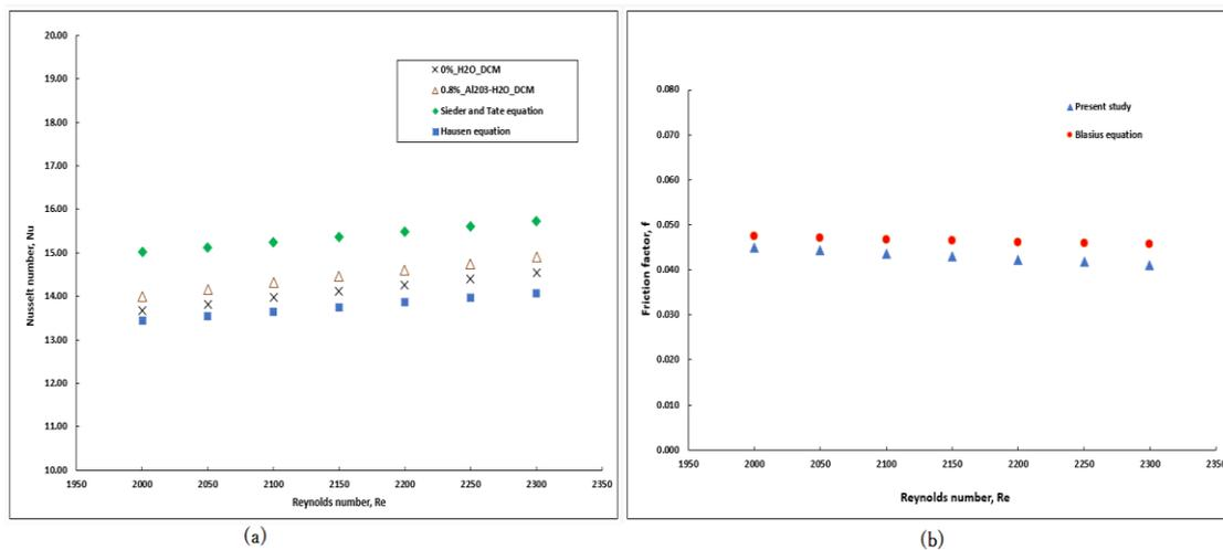
**Fig. 3** Validation of results of (a) Nusselt number and (b) friction factor as functions of Reynolds number
