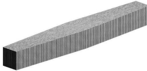
**Fig. 2.** 3D Mesh of the fluid domain
