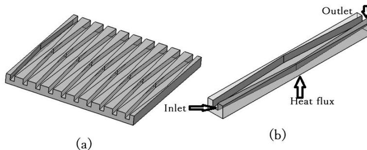
**Fig. 1** (a) 3D Schematic design of DCMCHS and (b) Computational domain
