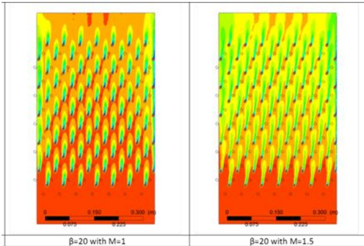
Fig. 17. Contour temperature for  $\beta = 20$
