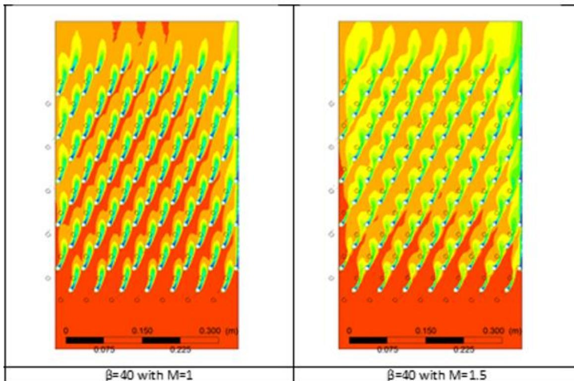
Fig. 19. Contour temperature for  $\beta = 40$
