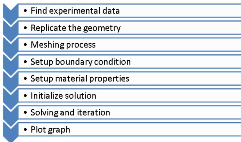
Fig. 1. Step in CFD process
