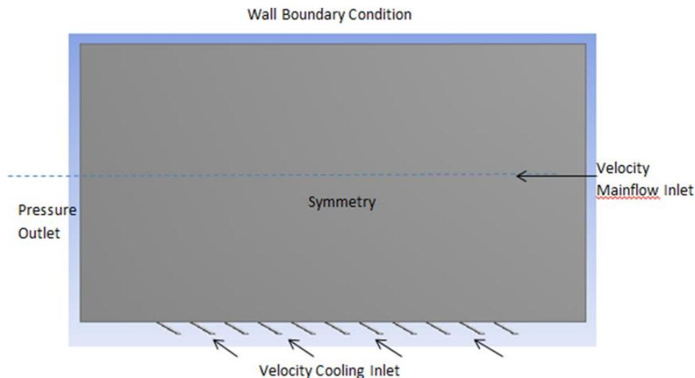
**Fig. 7.** Applied boundary condition on model
