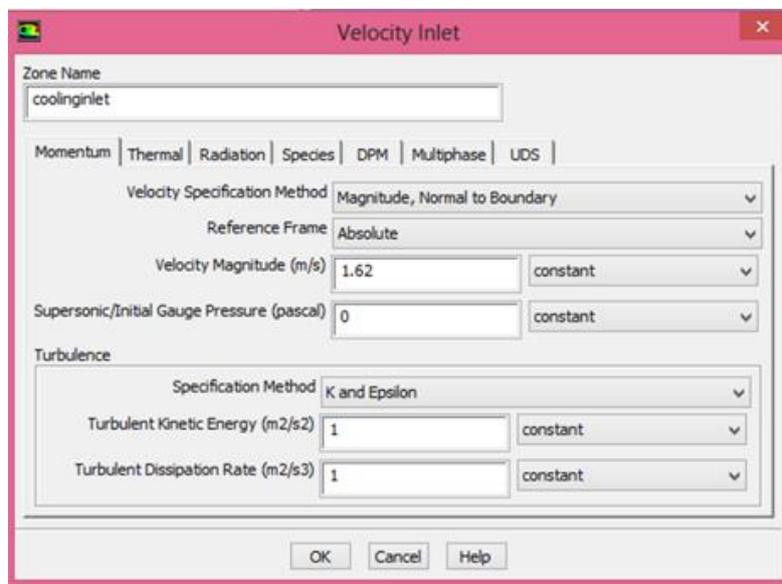
Fig. 12. Velocity profile for cooling inlet for M=1
