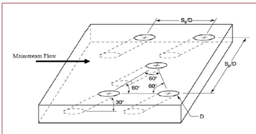
**Fig. 3.** The compound cooling hole arrangement
