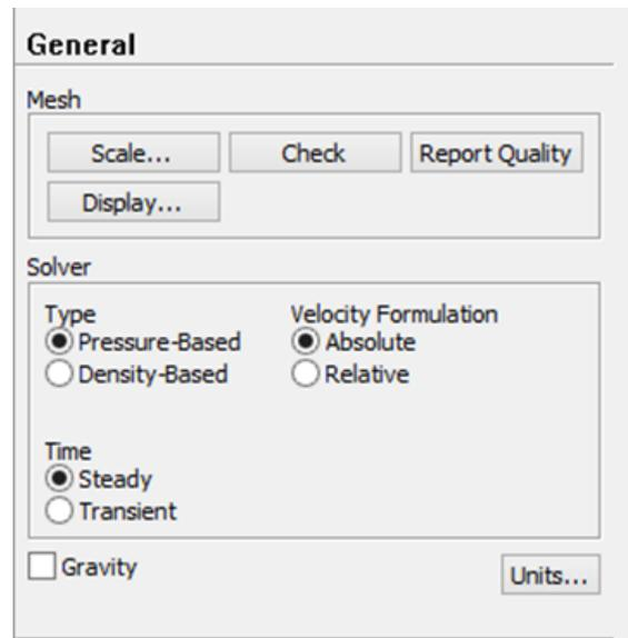
Fig. 9. The solver setting for fluent
