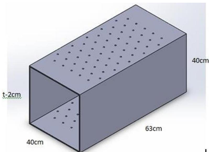
Fig. 2. Combustor model for simulator
