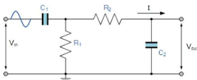
Fig. 1. An example of bandpass filter
