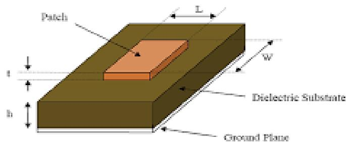
**Fig. 2.** Structure of a microstrip patch antenna
