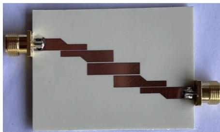
**Fig. 9.** Real fabricated design of BPF
