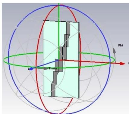
**Fig. 12.** 3D BPF design using CST
