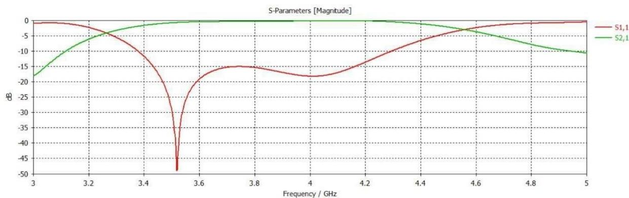
**Fig. 10.** Simulation results for S-Parameters using CST
