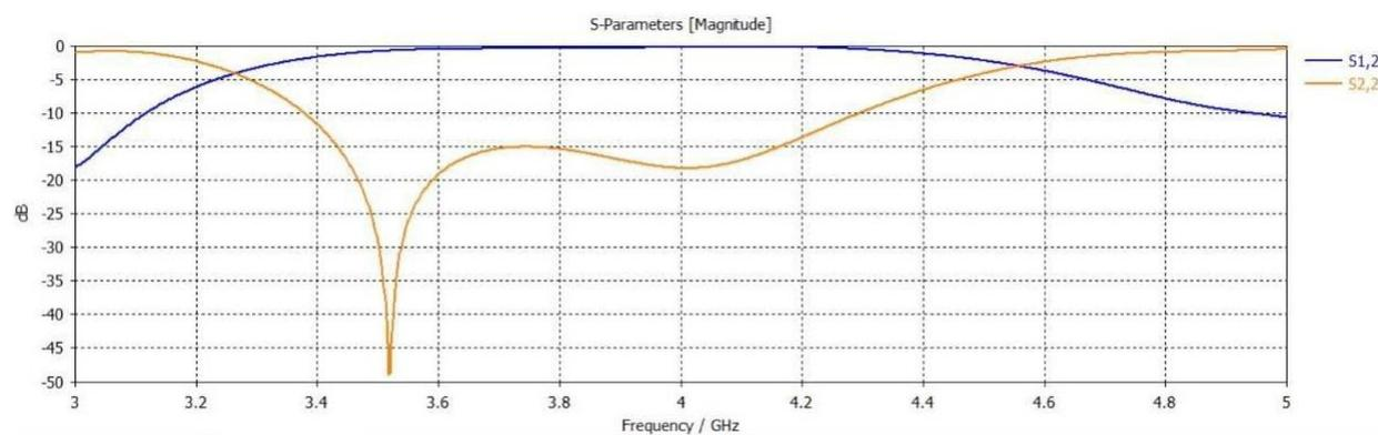
**Fig. 11.** Simulation results for S1,2 parameters using CST
