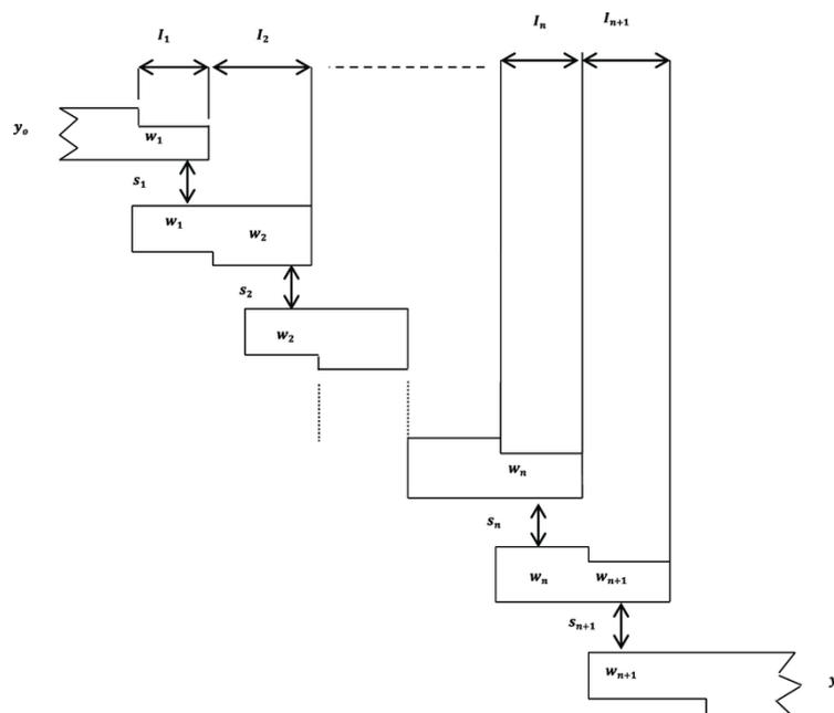
**Fig. 3.** General structure of parallel (edge)-coupled microstrip BPF
