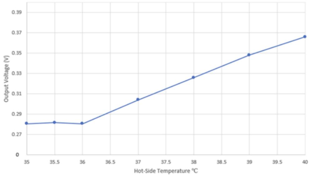
**Fig. 13.** Output voltage respected to hot side temperature
