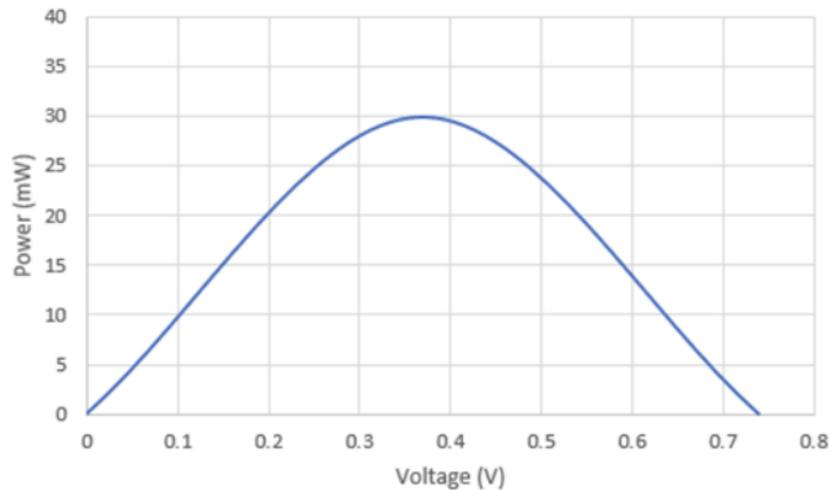
**Fig. 15.** Simulation result of output power respected to voltage at 40°C
