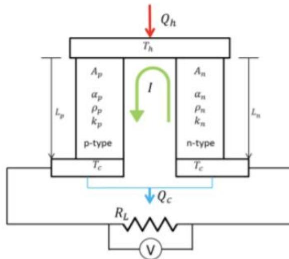
**Fig. 4.** TEG connected to a load
