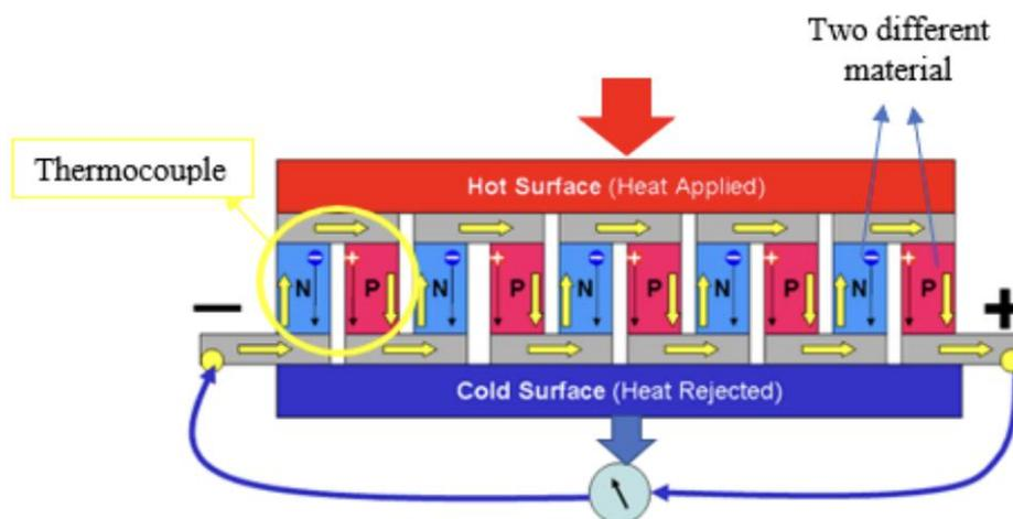
Fig. 2. Traditional TEG consists of N-type and P-type material [9]
