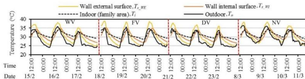
**Fig. 11.** The difference between surface temperature of exterior and interior wall with indoor temperature [16]
