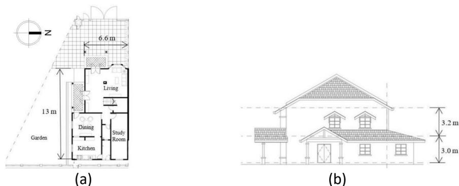
**Fig. 10.** The illustration of model two-storey terrace house (a) Ground floor plan and (b) Side view [16]
