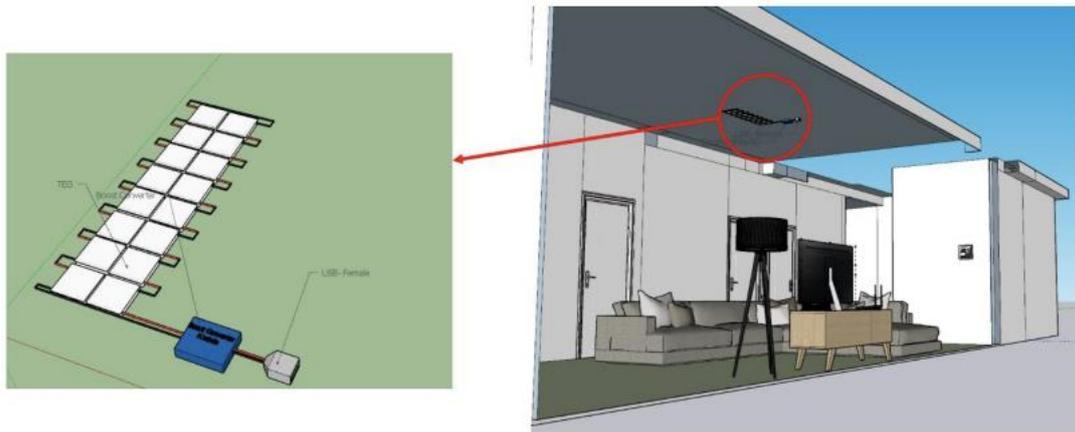
Fig. 20. A view of the TEG system to place in living room area
