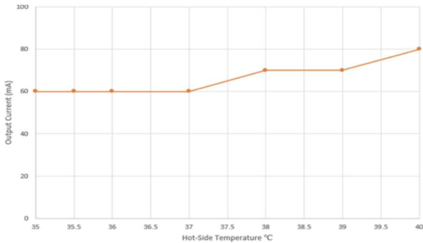
**Fig. 14.** Output current respected to hot side temperature
