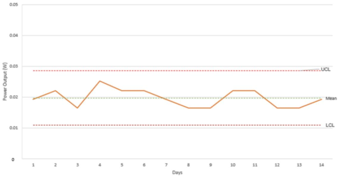
**Fig. 17.** Performance curve of TEM at external wall surface
