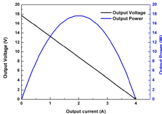
**Fig. 7.** I-V and I-W output characteristics of simulation data compare with manufacture data
