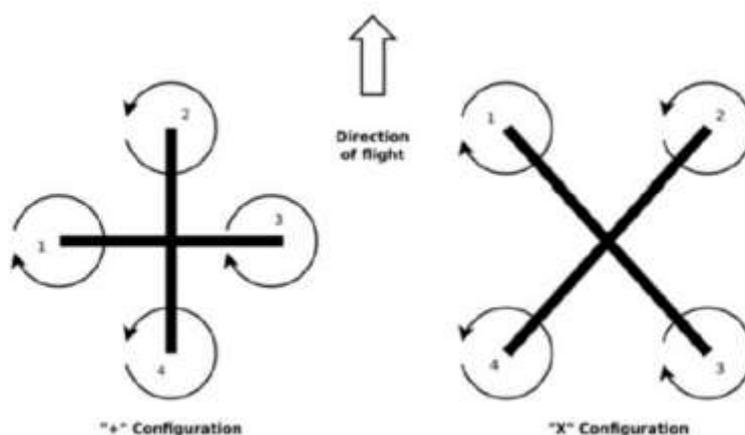
Fig. 1. Two main types of quadcopter configuration [3]
