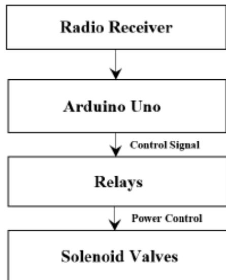
Fig. 2. Flowchart of control valves system
