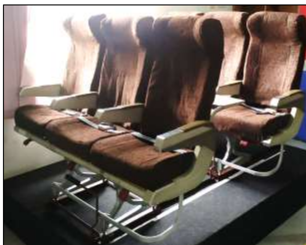
Fig. 2. Aircraft cabin mock-up used for the comfort experiment
