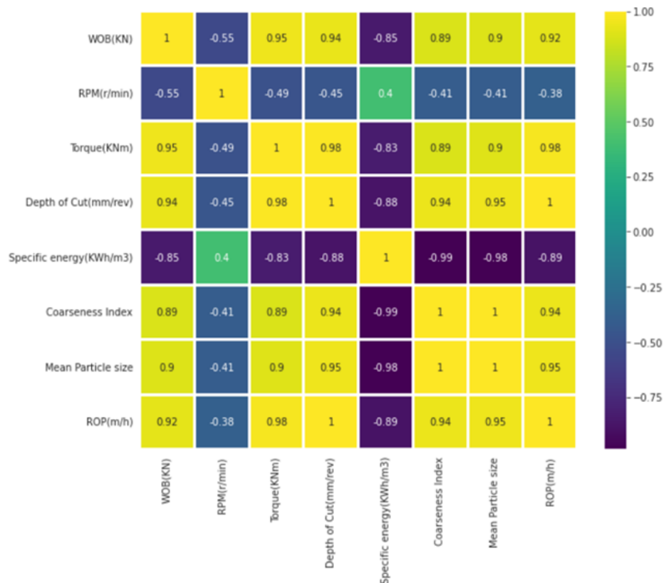
Fig. 2. Data visualization of the relationship between different drilling parameters by heatmap
