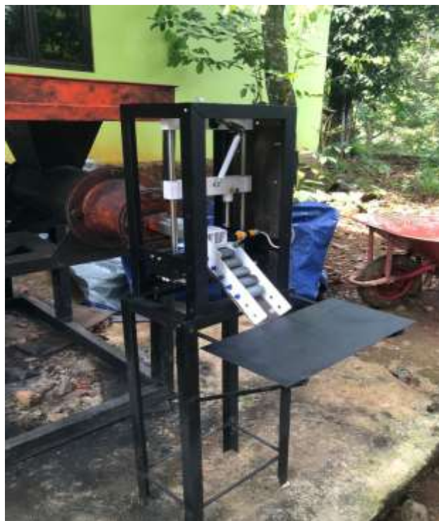
Fig. 10. Automated coconut shell charcoal briquette cutting tool performance test setups
