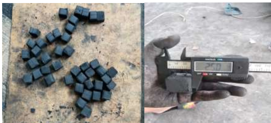
Fig. 11. Cube-shaped briquettes with a size of 2.5 x 2.5 x 2.5 cm
