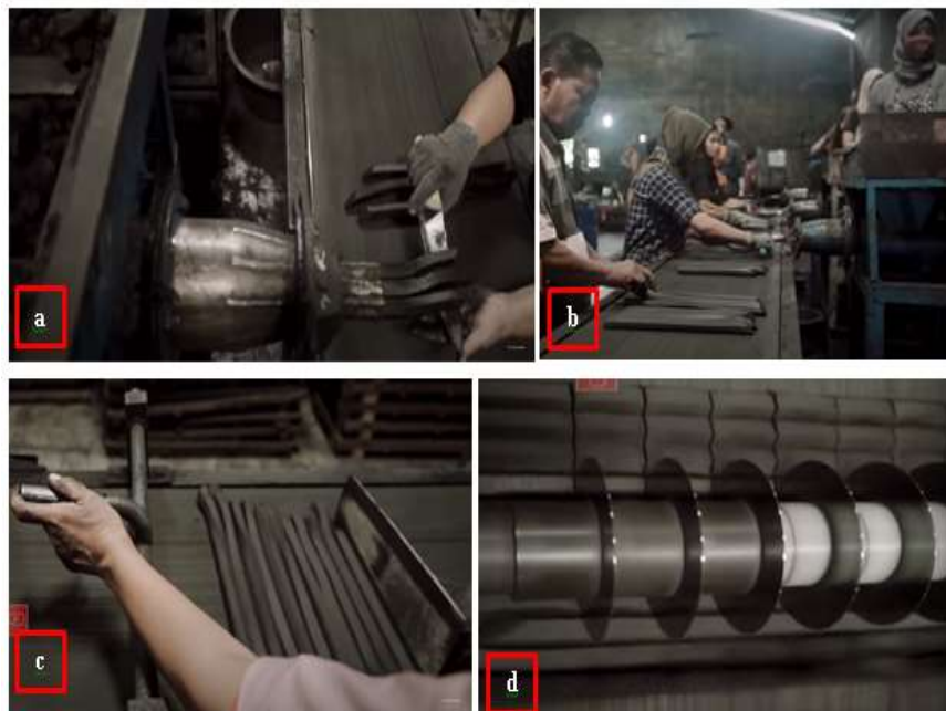
Fig. 1. Briquette cutting process using rotary cutting blades
