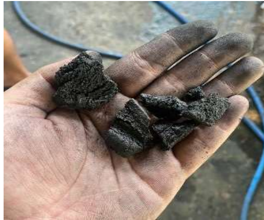
Fig. 12. Briquettes that are not cube-shaped
