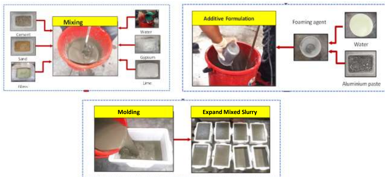
Fig. 1. The flow of the fabrication process of AAC-GIW
