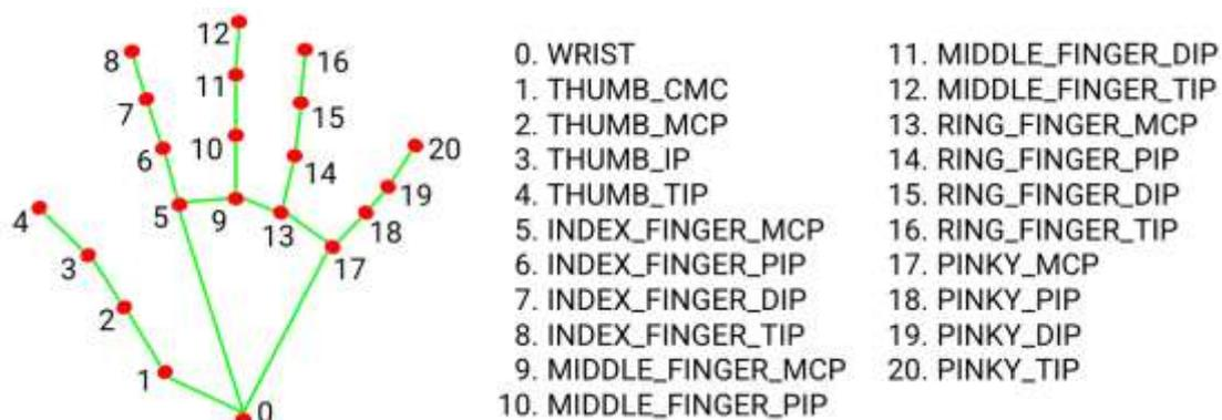
Fig. 3. MediaPipe's hand landmarks model [10]
