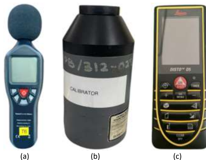
Fig. 1. (a) SLM25TK sound level meter (b) Acoustic calibrator (c) Laser meter
