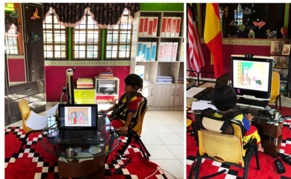
Fig. 5. The actual setup in the classroom. The T120 (in front of the participants) and the secondary screen (laptop) for the author to monitor the participant's eye fixations
