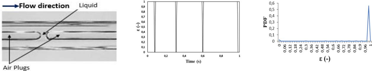
(a) Flow pattern (b) Void fraction time series (c) PDF
