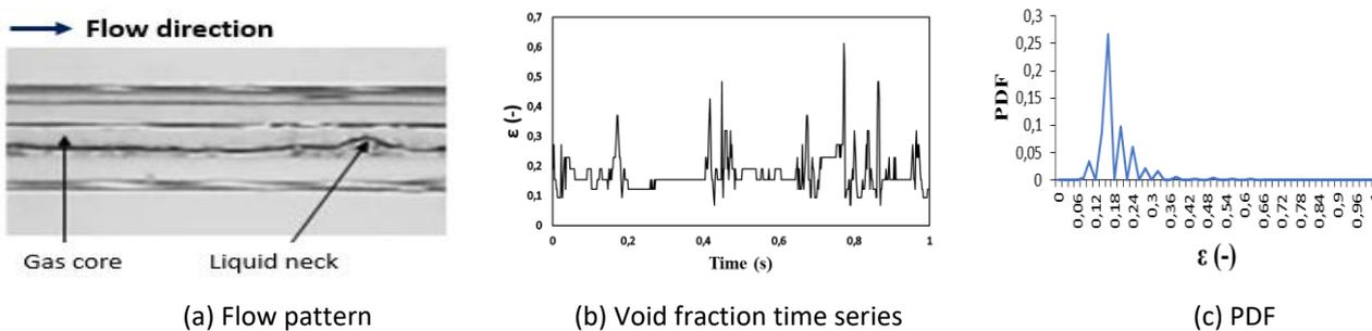
**Fig. 7.** Slug-annular flow at  $J_G = 3$  m/s and  $J_L = 0.033$  m/s for B3, 30° inclined orientation
