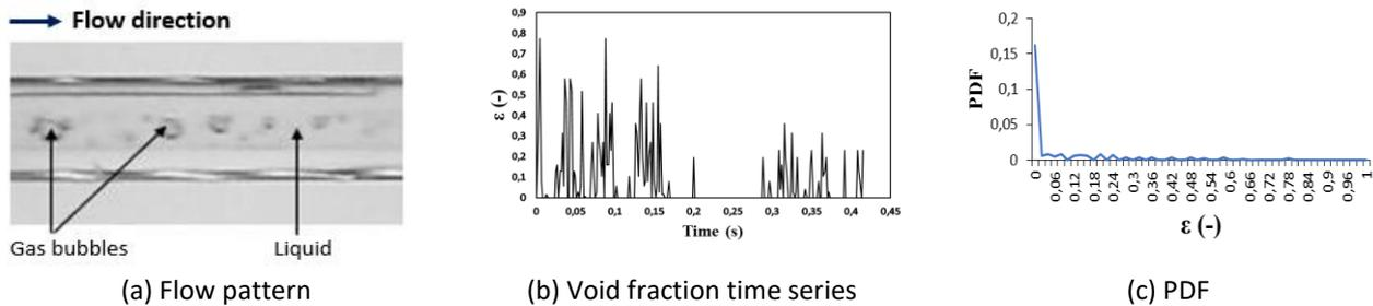
**Fig. 5.** Bubbly flow at  $J_G = 0.116$  m/s and  $J_L = 2.297$  m/s for B3, 30° inclined orientation
