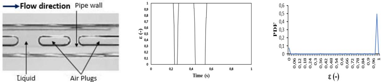
(a) Flow pattern (b) Void fraction time series (c) PDF
