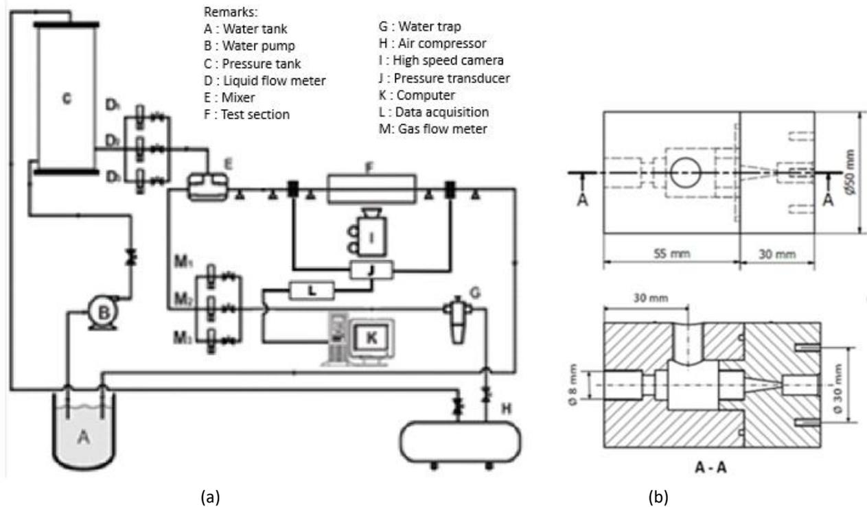
Fig. 1. (a) Schematic diagram of experimental apparatus, (b) mixer
