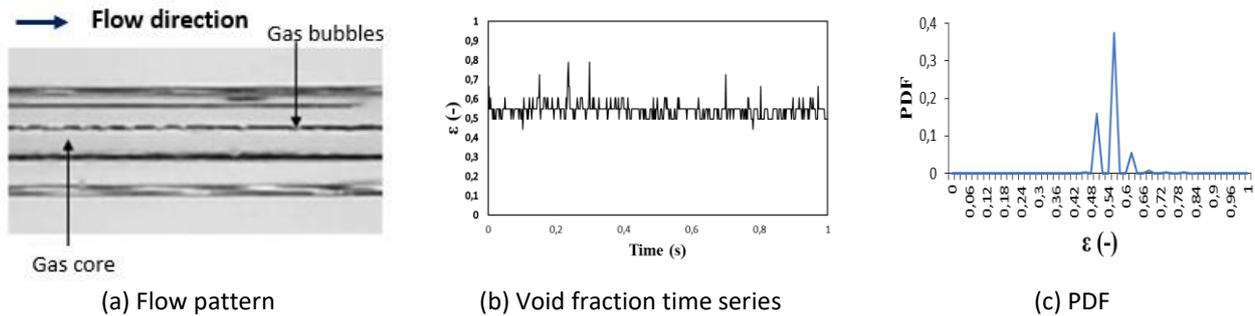
(a) Flow pattern (b) Void fraction time series (c) PDF
