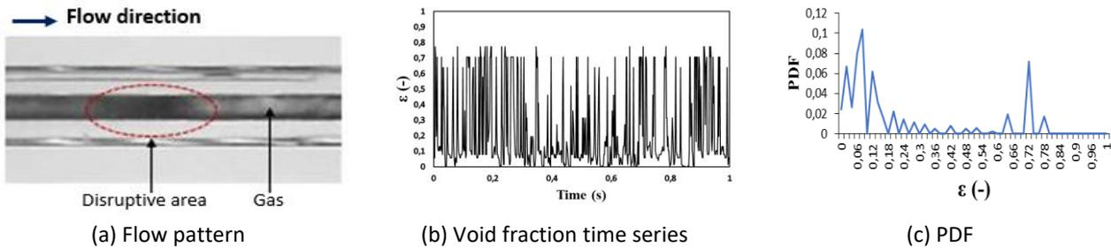
**Fig. 11.** Churn flow at  $J_G = 22.6$  m/s and  $J_L = 0.7$  m/s for B3,  $30^\circ$  inclined orientation
