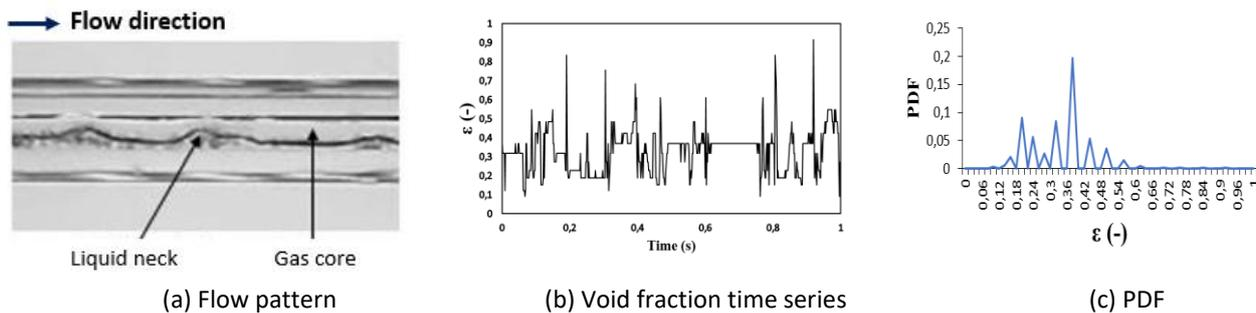
**Fig. 6.** Slug-annular flow at  $J_G = 3$  m/s and  $J_L = 0.0091$  m/s for B3, 30° inclined orientation
