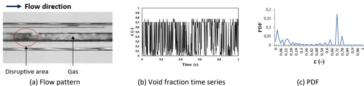
(a) Flow pattern (b) Void fraction time series (c) PDF
