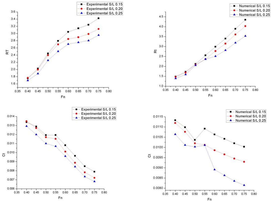
Fig. 5. The total resistance and total resistance coefficient of the model between experiment and numerical
