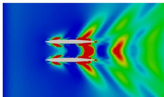
Fig. 4. Wave Pattern of the floats at Fn = 0.5
