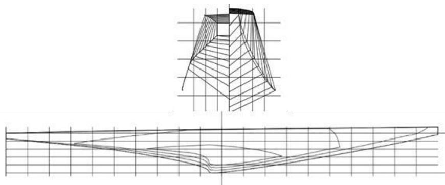
**Fig. 1.** Linesplan of the floats model
