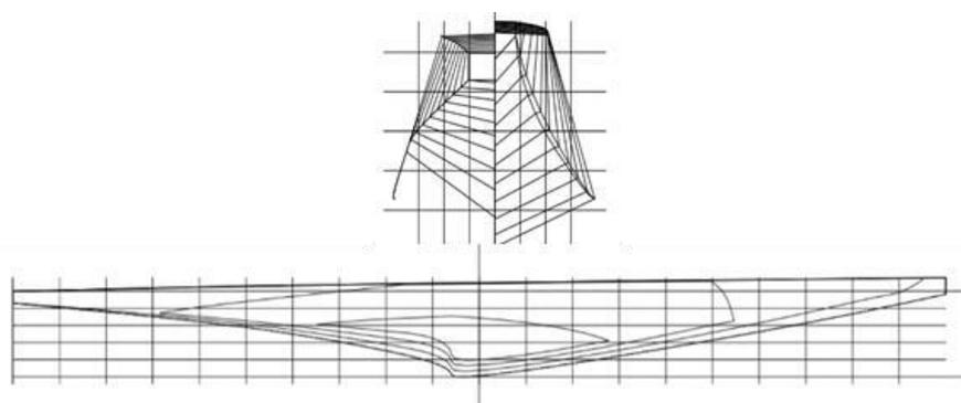
**Fig. 1.** Linesplan of the floats model
