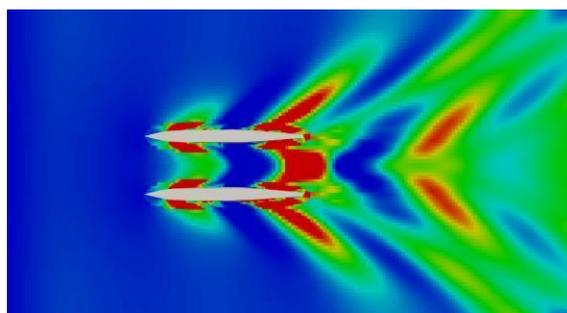
Fig. 3. Wave Pattern of the floats at Fn = 0.4
